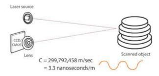
Figure 3 How the laser scanner works.
