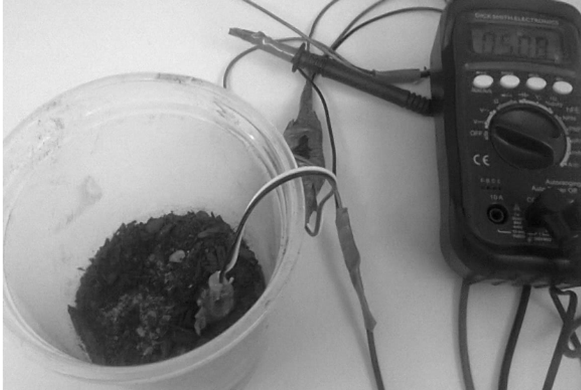
Figure 5.36: Undertaking Soil Moisture Probe Calibration
