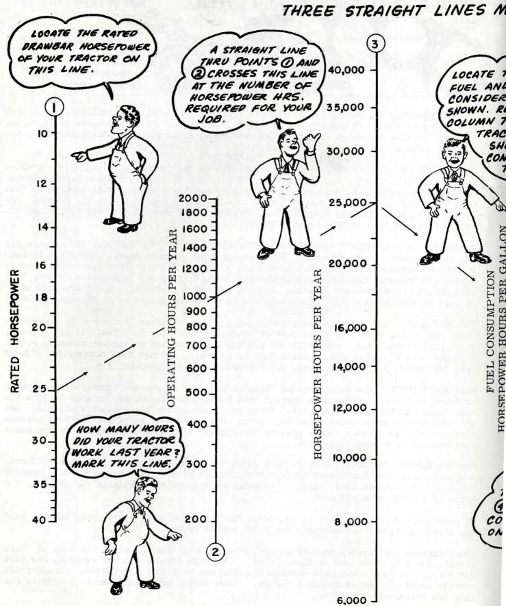
The horsepower hours per gallon shown for different fuels on line 4 are average These are for whee from tests on current tractors tested prior to 1954. tractors on the ten hour drawbar test. For power units and tracklayers, see in formation on the front of this folder.
