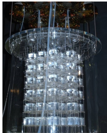
Figure 2. Picture of 96 \text{CaF}_2 crystals used in CANDLES.
