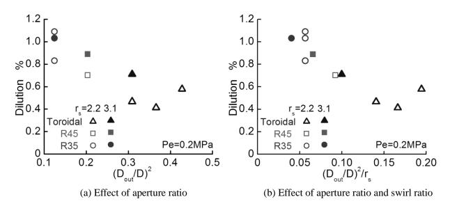
Fig.11. Effect of gas velocity on fuel dilution.(a) Effect of aperture ratio. (b) Effect of aperture ratio and swirl ratio.
