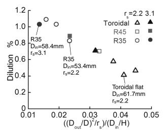
Fig.12. Effect of gas flow on fuel dilution.
