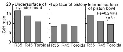
Fig.8. Elementary analysis (C/H ratio) of deposit.
