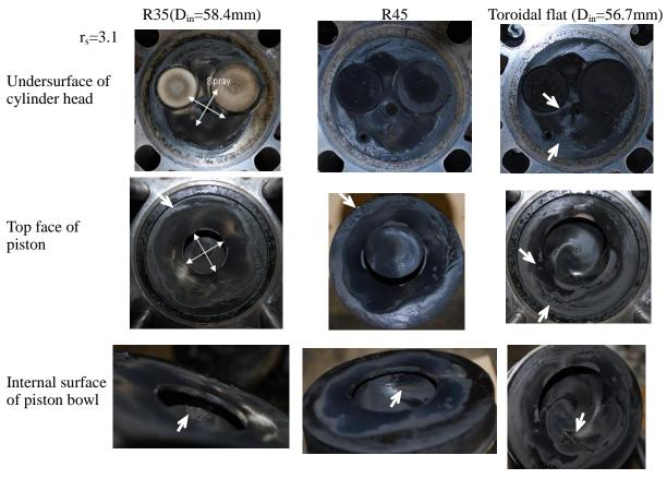
Fig.6. Deposit formation on the wall surface.
