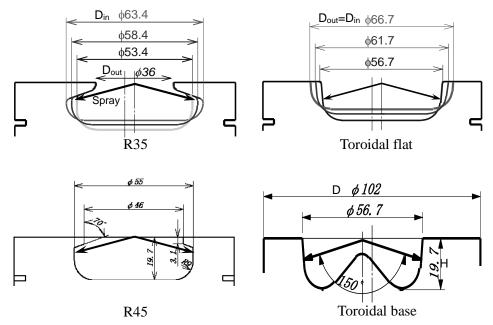
Fig.3. Piston configurations.
