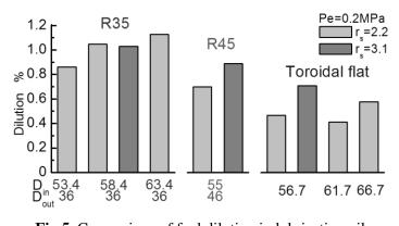
Fig.5. Comparison of fuel dilution in lubricating oil.
