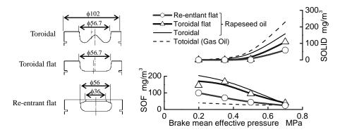
Fig.1. Reduction of particulate emissions by means of combustion chamber configurations [26].
