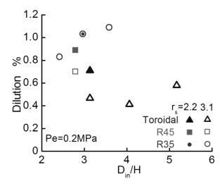
Fig.10. Relation between aspect ratio and fuel dilution in lubricating oil.
