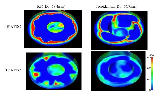
Fig.7. CFD analysis of fuel distribution near the top surface of piston.
