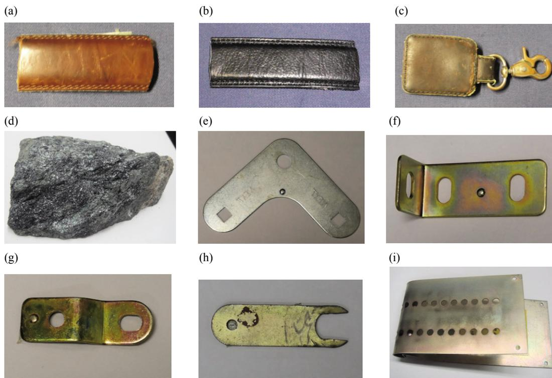
**Fig.1** Photographs of chromium-containing samples analyzed. (a) leather 1, (b) leather 2, (c) leather 3, (d) mineral (fuchsite: green muscovite mica), (e) bracket 1, (f) bracket 2, (g) bracket 3, (h) old wrench and (i) electronic device chassis.
