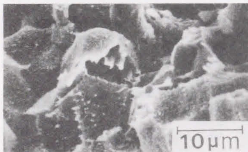
Fig. 2-15 SEM Photograph of Calcium Silicate Hydrate Autoclaved at 200^\circ\text{C} for 10h Used \text{NaOH} 15% Solution ( \text{CaO}/\text{SiO}_2=0.40 )
