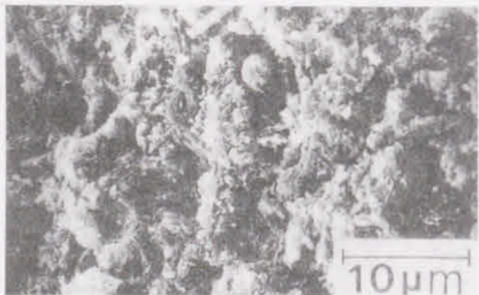
Fig. 2-13 SEM Photograph of Calcium Silicate Hydrate Autoclaved at 200°C for 10h (CaO/SiO 2 =0.40)
