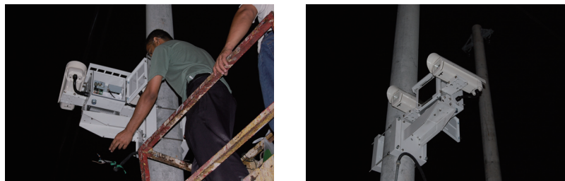
Figure 2.4 High Speed camera with strong IR probe
