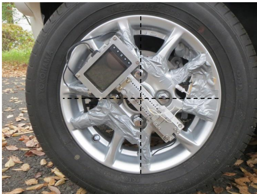
Fig. 5.29. Apparatus for the actual-vehicle experiment of centrifugal force effect under the position of rotating center.
