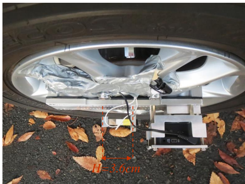
Fig. 5.33. Apparatus for the actual-vehicle experiment of linear system under the centrifugal position of 3.6 cm.
