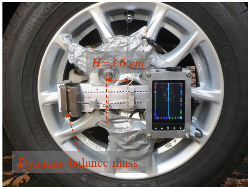
Fig. 5.31. Apparatus for the actual-vehicle experiment of centrifugal force effect under the centrifugal position of 3.6 cm.
