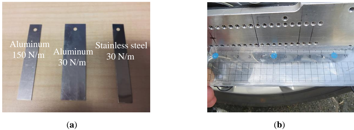
Fig. 5.26. (a) Different types of beams for tire rotating experiments; (b) Determination of the centrifugal distances.
