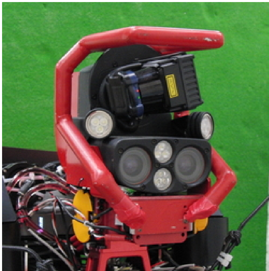
Fig 11: Vision sensor for JAXON(Carnegie Robotics MultiSense SL).[104]
