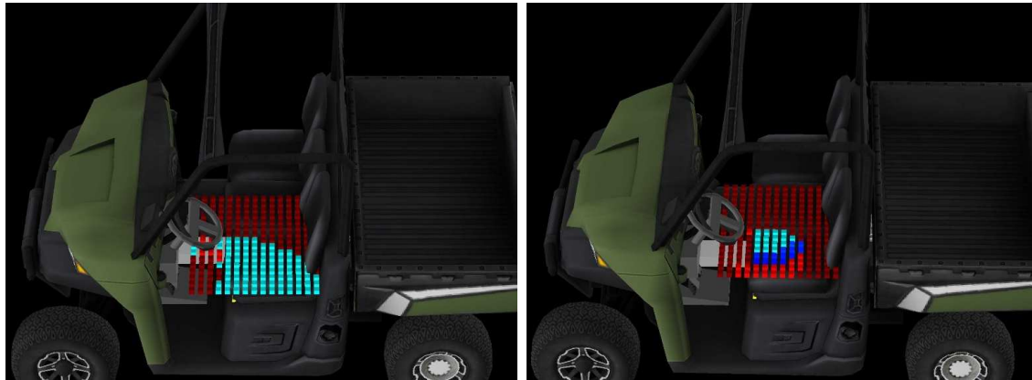
Fig 5.6: Manipulable region of steering for JAXON(left) and HRP2(right) by left arm. The sitting position where the robot can turn 360[deg] is light blue, one where the robot can grasp a crank but cannot turn 360[deg] is deep blue, and one where the robot cannot grasp crank is red
