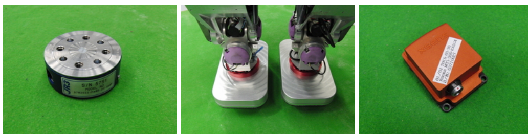
Fig 9: Main sensors in JAXON: 6-axis force sensor(JR3 67M25S3-M40B-DH), 6-axis force plate(Leptrino CFP230QA202R), IMU(Xsens MTi-300-6A5G4).[104]
