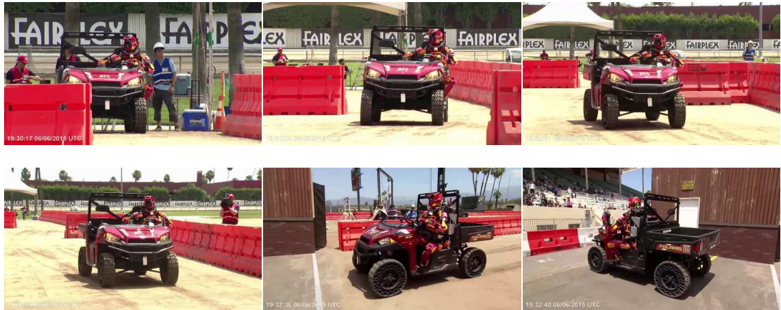
Fig 5.14: JAXON drives a vehicle in DARPA Robotics Challenge[99] (time series from upper left to lower right)[80]
