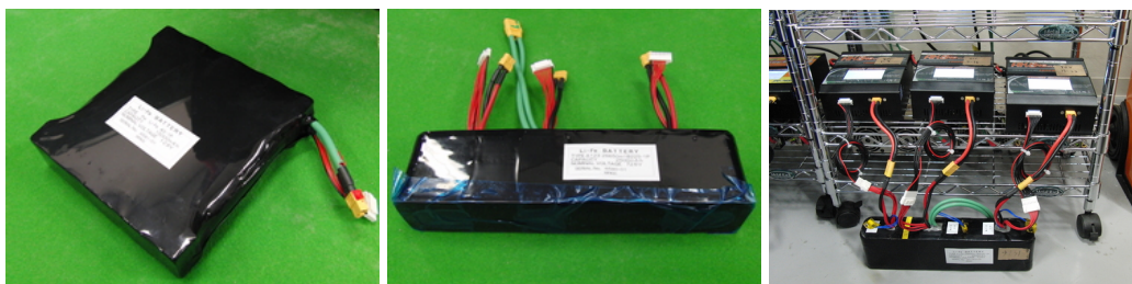
Fig 7: 12V Line Li-Fe Battery, 80V Line Li-Fe Battery and Charging Station (left to right)[104]
