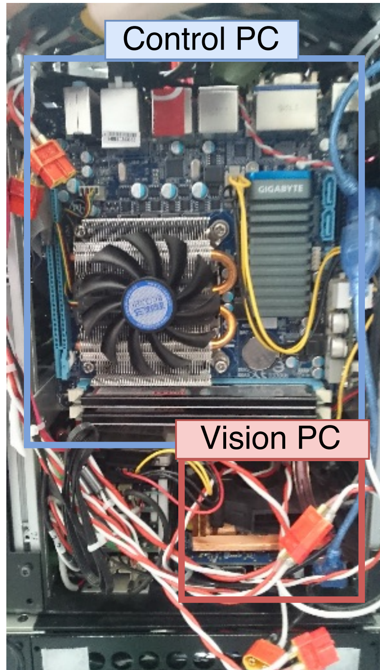
Fig 12: Control PC and Vision PC inside Robot back pack[104]
