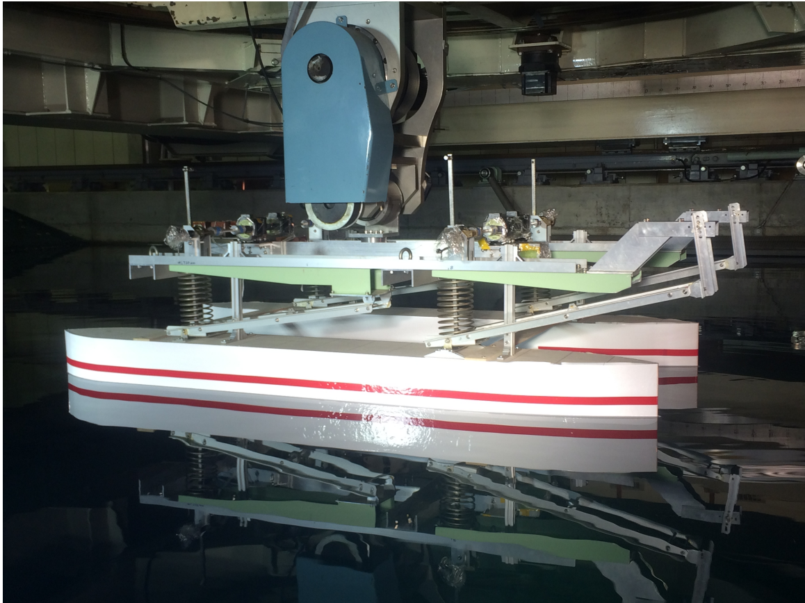
Figure A.8: Experimental setup of the hydrodynamic test in a towing tank
