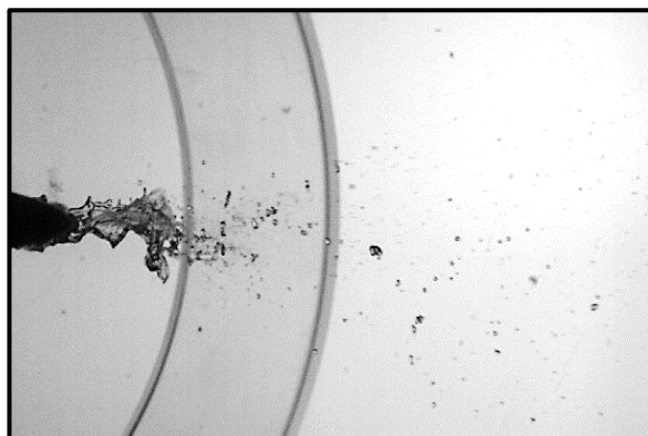
(i) Disintegration of water from T.E. (131 m.sec)
