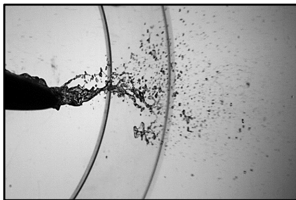
(k) Disintegration of large chunk of accumulated water (176.33 m.sec)
