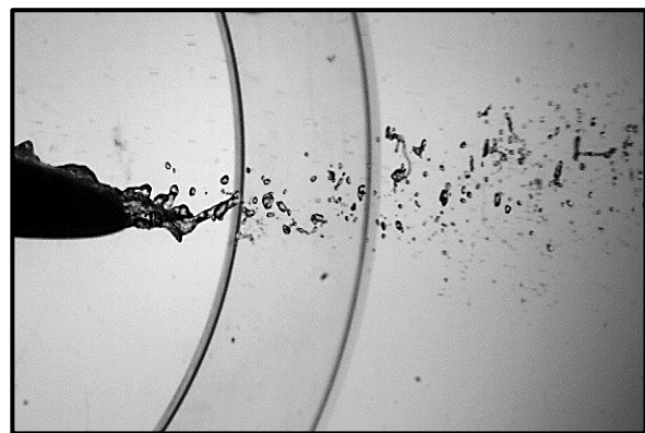
(l) Fine & Coarse Droplets in Karman Vortex Street (176.66 m.sec)
