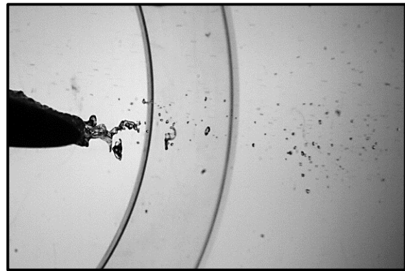
(h) Stripping of droplets from T.E. (75.66 m.sec)
