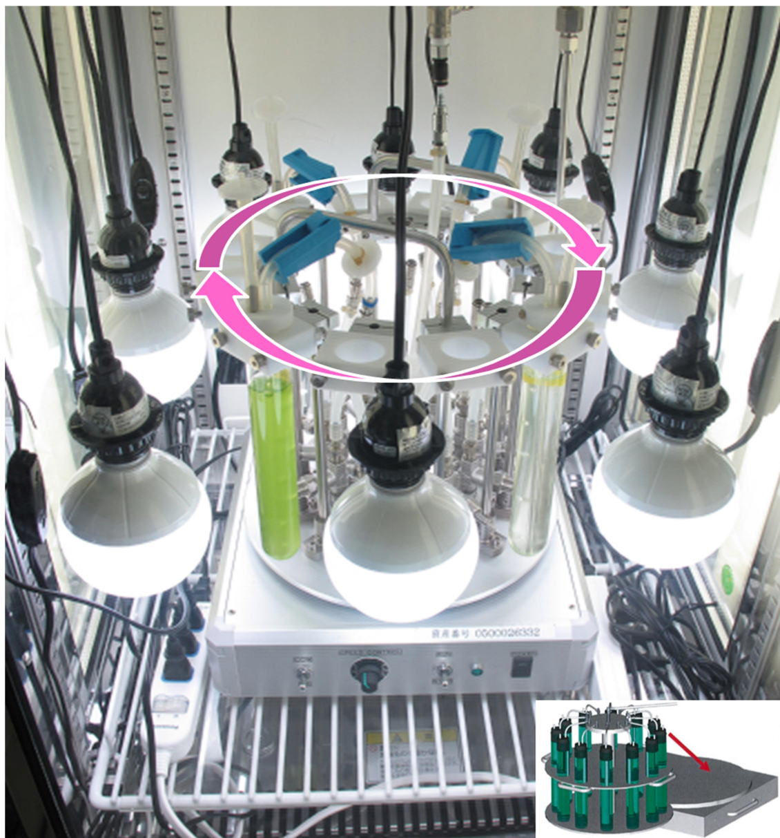
Fig. 2–S1. Rotary culture equipment. Cultivation was performed in a maximum of 12 test tubes fixed to a central platform holder, which was rotated at 2 rpm.
