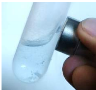
図 3.10: Liquid oxygen attracted by the magnet.
