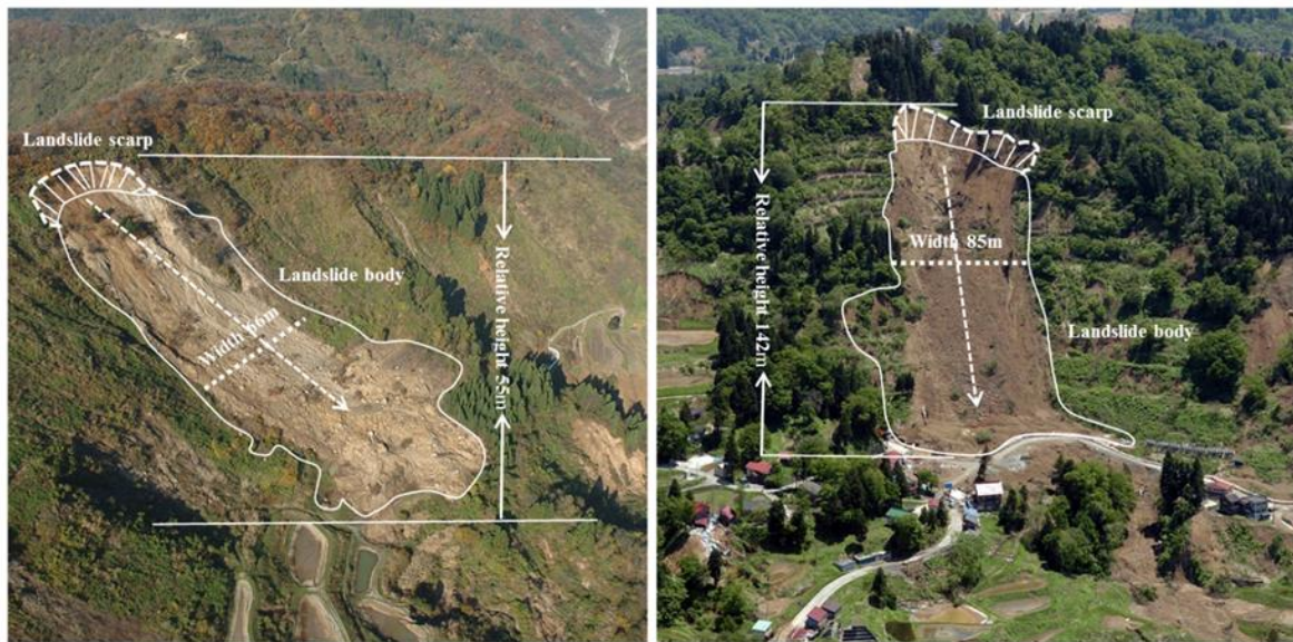
Figure 2-5 A shallow landslide (left) in the southwest of Nigorizawa, Nagaoka City; and a deep-seated (right) landslide in the western entrance of the Haguro tunnel, Nagaoka City. Width and relative height for the deep-seated landslide is larger than those of the shallow landslides. (Images provided by NIED).
