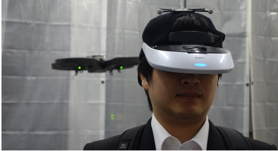
Figure 3.1: FlyingHead is a telepresence system that remotely connects humans and unmanned aerial vehicles (UAVs). The system synchronizes the operator’s head motions with the UAV’s movement and it enables the operator to experiences augmented abilities as if he or she become a flying robot.
