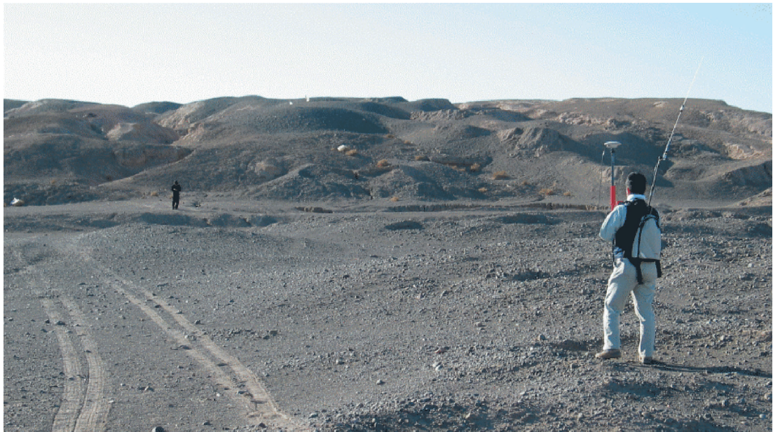
Fig. 2. The Bam scarp (Bam fault) southwest of Baravat village at the Loc. 4 in the report by Okumura et al. (See the text in this volume). Here the scarp is about 15m high and partly buried with recent alluvial fan deposit from a stream cutting into the scarp. Members of the post-earthquake survey are measuring the profile of the scarp with RTK-GPS. Photograph by Koji Okumura on January 31st, 2004.
