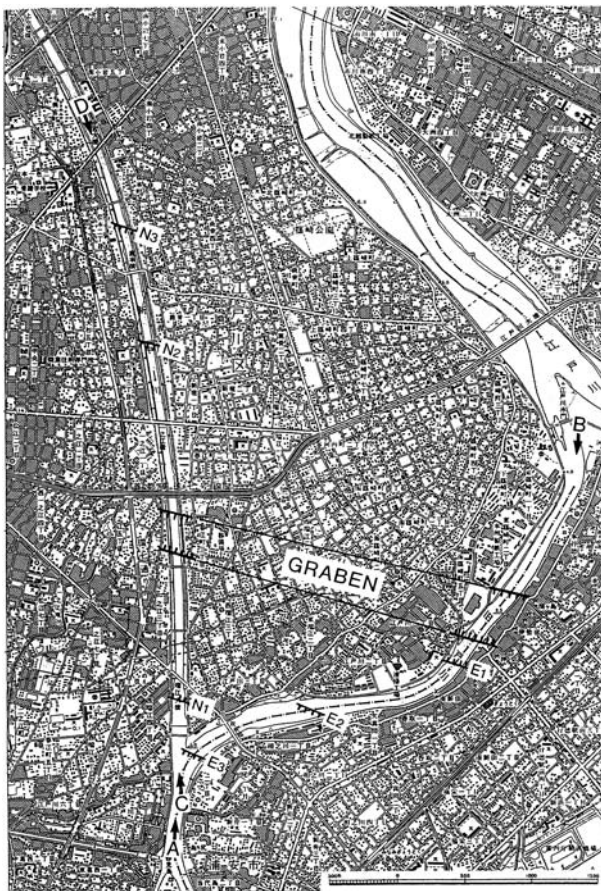
Fig. 7. Lines of multi-channel seismic profiling survey (A-B and C-D) and location of graben structure. E1-E3 and N1-N3 indicate the location of faults (from Sugiyama and Endo, 1993).
