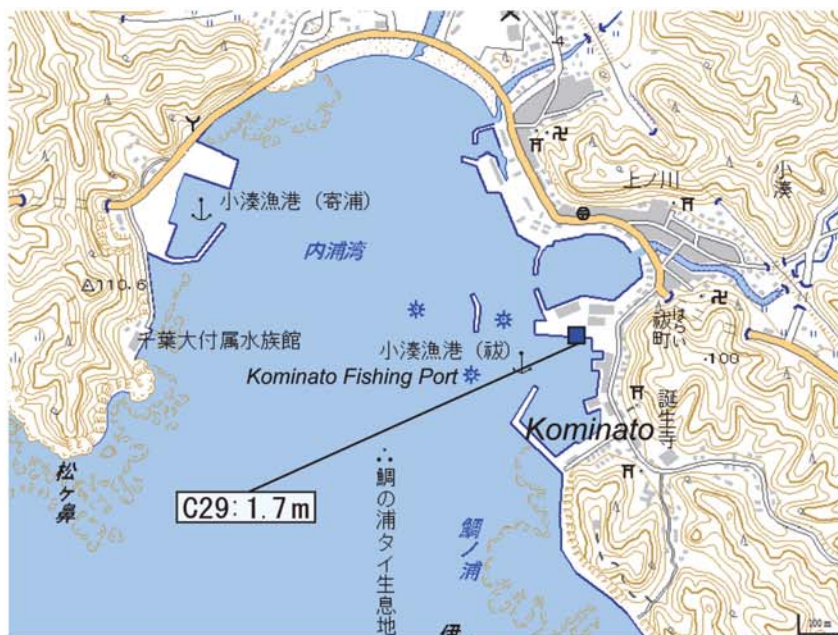
Fig. A333. Tsunami height at Kominato (Kominato Fishing Port), Kamogawa City, Chiba Prefecture (added with a digital topographic map at a scale of 1/25,000 from the Geospatial Information Authority of Japan). The symbol and its meaning are the same as in Fig. 6.
