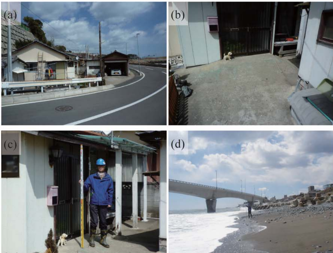
Fig. A264. (a) Mr. Seya's house in Higashicho (tsunami trace survey point). (b) Tsunami inundated near the entrance sliding doors. (c) Tsunami trace survey point in front of the entrance doors of Mr. Seya's house (B18). (d) Measuring ground height at a survey point based on the water surface of sea.
