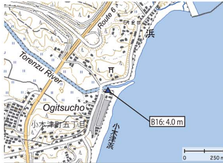
Fig. A259. Tsunami height at Ogitsucho, Hitachi City, Ibaraki Prefecture (added with a digital topographic map at a scale of 1/25,000 from the Geospatial Information Authority of Japan). The symbol and its meaning are the same as in Fig. 5.
