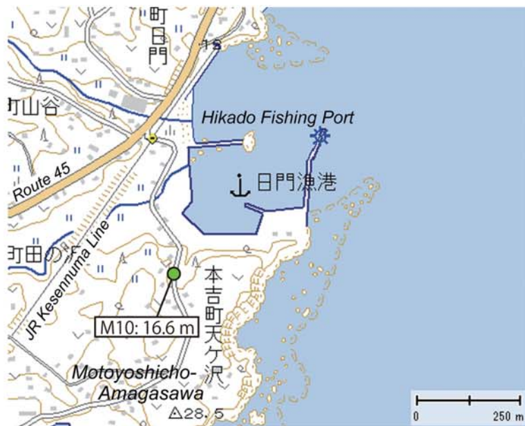
Fig. A145. Tsunami height at Motoyoshicho-Amagasawa (Hikado Fishing Port), Kesenuma City, Miyagi Prefecture (added with a digital topographic map at a scale of 1/25,000 from the Geospatial Information Authority of Japan). The symbol and its meaning are the same as in Fig. 4.
