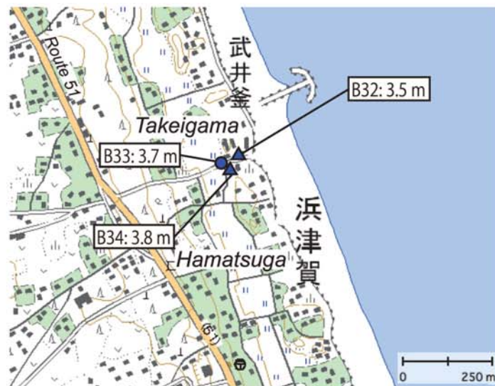
Fig. A285. Tsunami heights at Takeigama (B32 and B33) and Hamatsuga (B34), Kashima City, Ibaraki Prefecture (added with a digital topographic map at a scale of 1/25,000 from the Geospatial Information Authority of Japan). The symbols and their meanings are the same as in Fig. 5.
