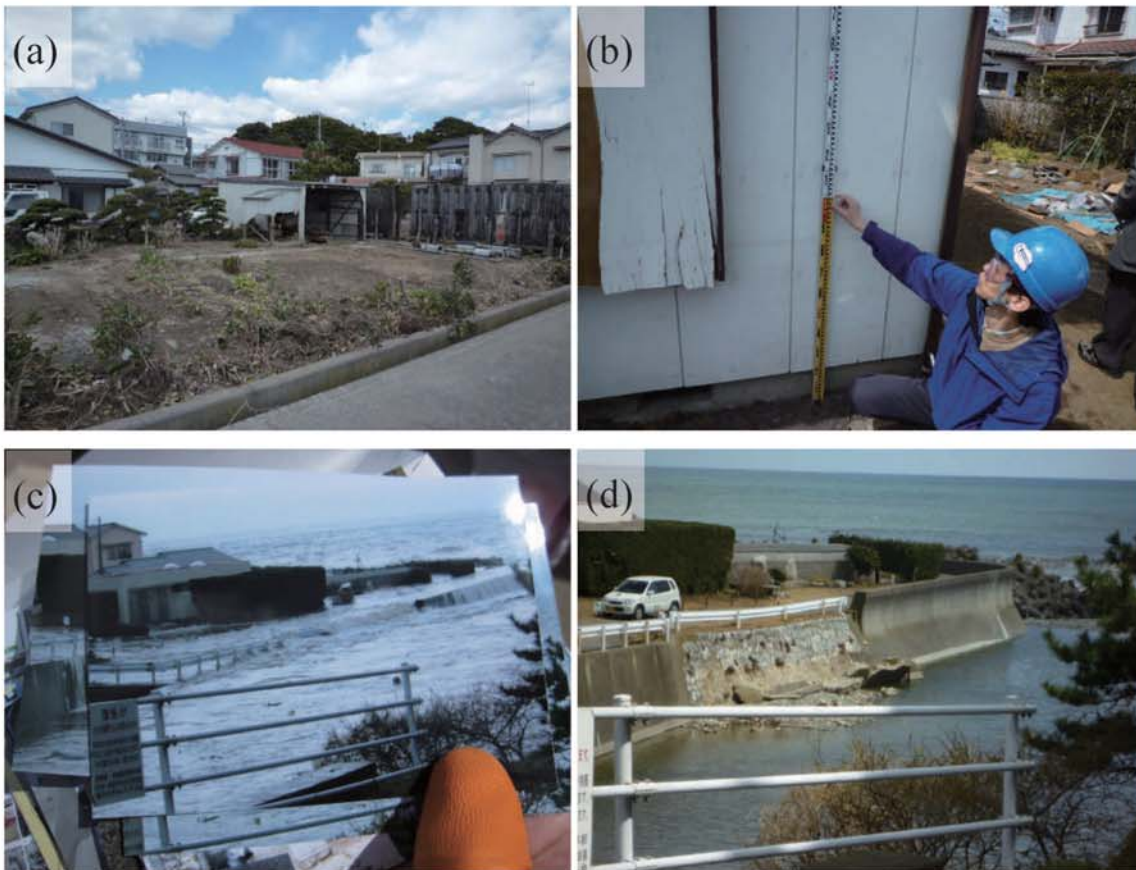
Fig. A268. (a) Mr. Shimazaki's house damaged by the tsunami (tsunami trace survey point). (b) Watermark on a wall of Mr. Shimazaki's house (1.01 m above ground level, B20). (c) Photographs taken by Mr. Shimazaki show that the tsunami flowed over the top of the seawall around his house (B21). (d) Seawall shown in Mr. Shimazaki's photograph.
