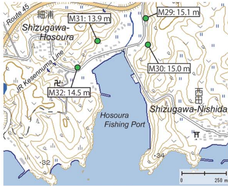
Fig. A167. Tsunami heights at Shizugawa-Nishida (M29 and M30) and Shizugawa-Hosoura, (M31 and M32) Minamisanriku Town, Miyagi Prefecture (added with a digital topographic map at a scale of 1/25,000 from the Geospatial Information Authority of Japan). The symbols and their meanings are the same as in Fig. 4.
