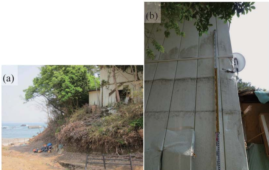
Fig. A138. (a) Damage at Karakuwacho-Kakehama. (b) Tsunami trace survey point on a wall of a house on the southern slope (2.85 m above ground level, M3).
