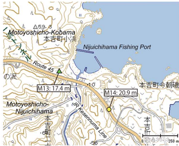
Fig. A151. Tsunami heights at Motoyoshicho-Nijuichihama, Kesenuma City, Miyagi Prefecture (added with a digital topographic map at a scale of 1/25,000 from the Geospatial Information Authority of Japan). The symbols and their meanings are the same as in Fig. 4.
