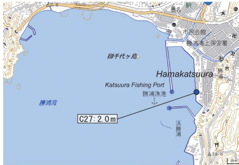
Fig. A329. Tsunami height at Hamakatsuura (Katsuura Fishing Port), Katsuura City, Chiba Prefecture (added with a digital topographic map at a scale of 1/25,000 from the Geospatial Information Authority of Japan). The symbol and its meaning are the same as in Fig. 6.
