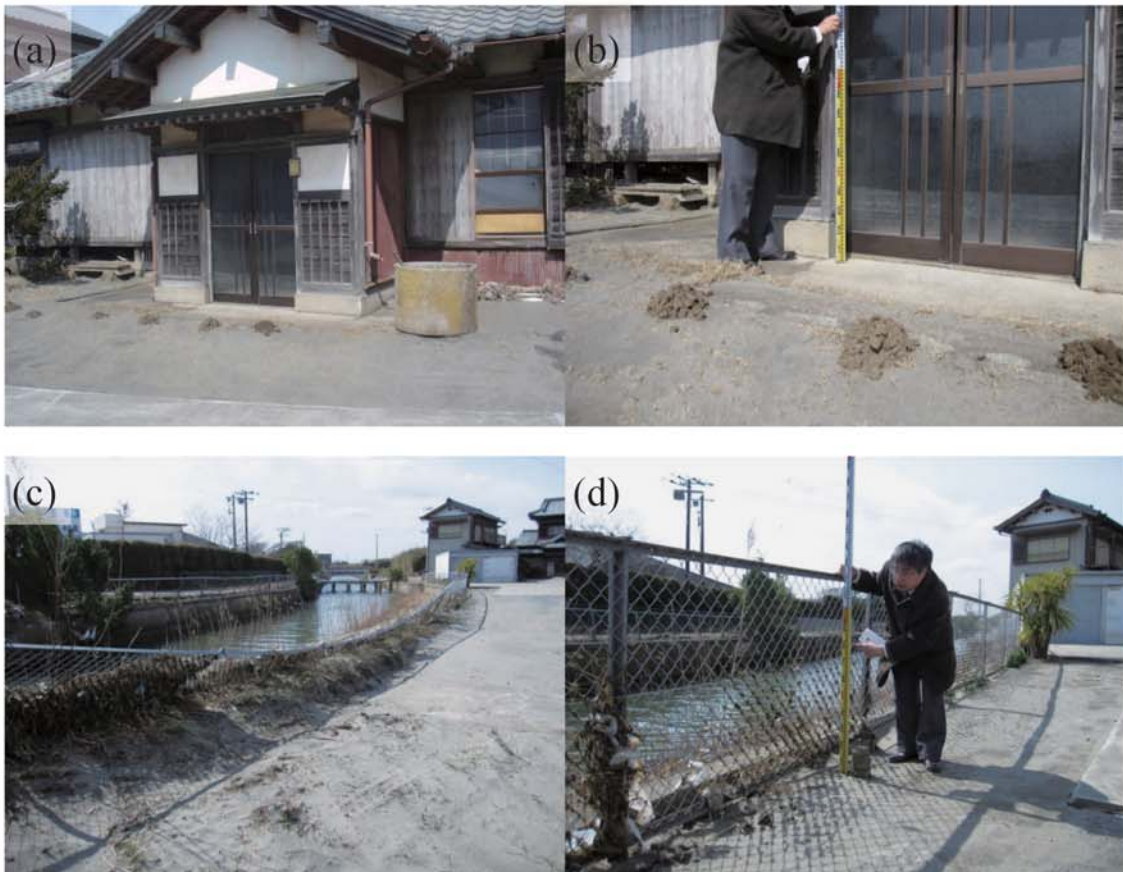
Fig. A306. (a)-(b) Watermark on the entrance sliding doors of Mr. Ui's house near the Niibori River (0.37 m above ground level; C9). (c)-(d) Glass and see glass attached to a fence along the Niibori River (0.76 m above ground level; C10).
