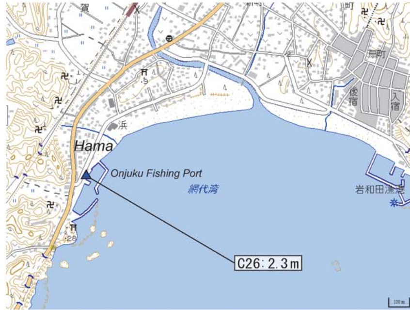
Fig. A327. Tsunami height at Hama (Onjuku Fishing Port), Onjuku Town, Chiba Prefecture (added with a digital topographic map at a scale of 1/25,000 from the Geospatial Information Authority of Japan). The symbol and its meaning are the same as in Fig. 3.
