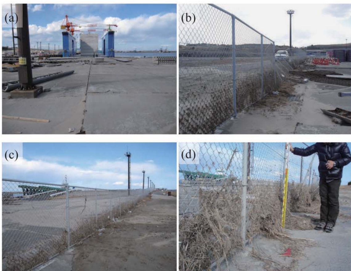
Fig. A276. (a) Ibaraki Port Hitachinaka District (Hitachinaka Port). (b) Damage at Hitachinaka Port. (c) Dry grass on a fence at the port. (d) Measuring height of average upper end of dry grass caught on the fence as the tsunami inundation height (1.03 m above ground level, B26).
