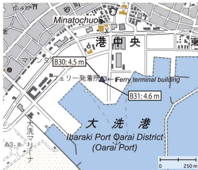
Fig. A283. Tsunami heights at Minatocho (Ibaraki Port Oarai District), Oarai Town, Ibaraki Prefecture (added with a digital topographic map at a scale of 1/25,000 from the Geospatial Information Authority of Japan). The symbols and their meanings are the same as in Fig. 5.
