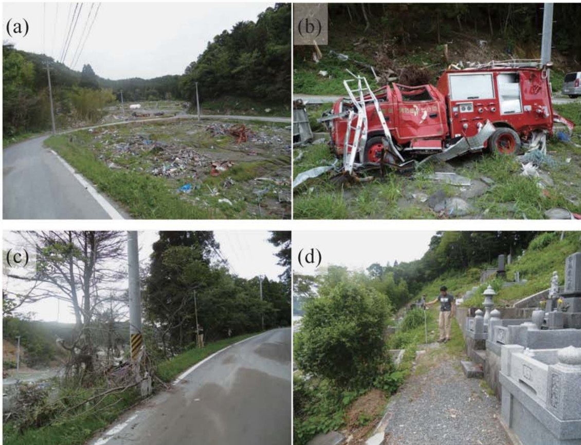
Fig. A224. (a)-(b) Damage at Yagawahama. (c) Tsunami trace survey point on a tree on the eastern slope (2.80 m above ground level, M67). (d) Tsunami trace survey point at a grave site beside the temple Dofukudera (M68).
