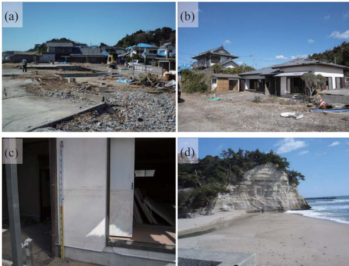
Fig. A260. (a) Damage near the mouth of the Torenzu River in Ogitsucho. (b) Mr. Ikutame's house damaged by tsunami (tsunami trace survey point). (c) Watermark on a wall of Mr. Ikutame's house (1.34 m above ground level, B16). (d) Measuring ground height at the survey point based on water surface in the Torenzu River.
