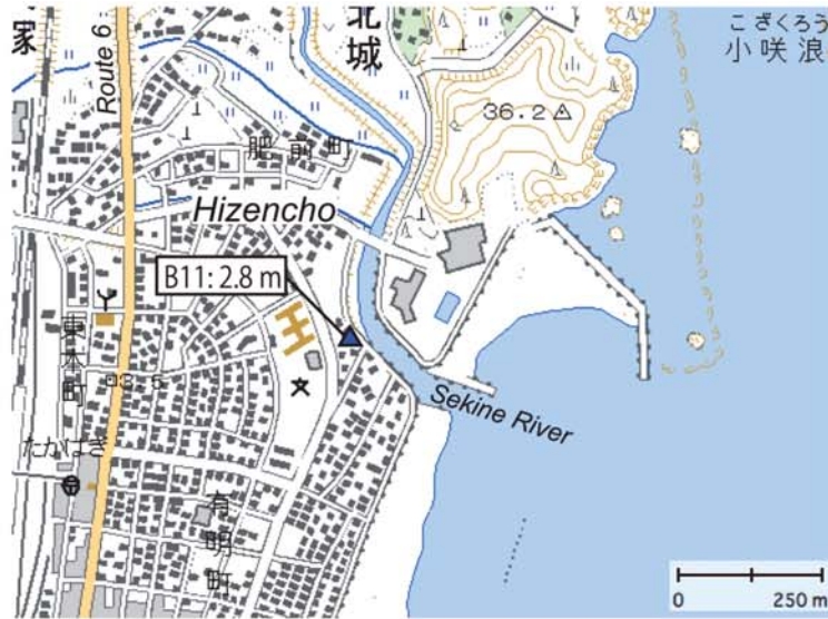
Fig. A251. Tsunami height at Hizencho, Takahagi City, Ibaraki Prefecture (added with a digital topographic map at a scale of 1/25,000 from the Geospatial Information Authority of Japan). The symbol and its meaning are the same as in Fig. 5.
