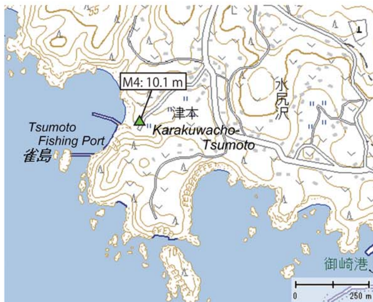
Fig. A139. Tsunami height at Karakuwacho-Tsumoto, Kesennuma City, Miyagi Prefecture (added with a digital topographic map at a scale of 1/25,000 from the Geospatial Information Authority of Japan). The symbol and its meaning are the same as in Fig. 4.
