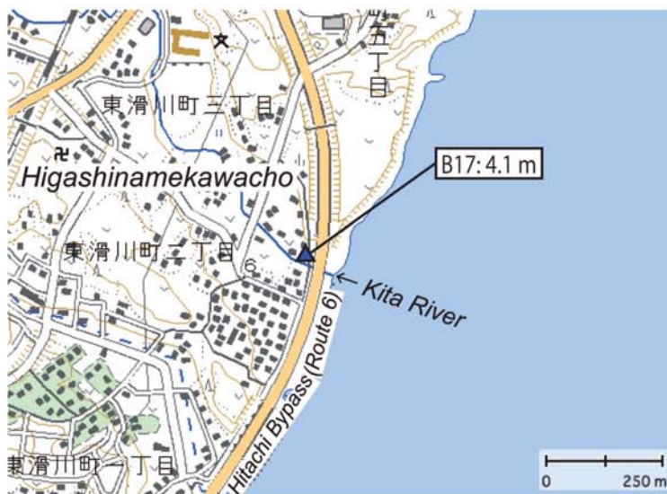
Fig. A261. Tsunami height at Higashinamekawacho, Hitachi City, Ibaraki Prefecture (added with a digital topographic map at a scale of 1/25,000 from the Geospatial Information Authority of Japan). The symbol and its meaning are the same as in Fig. 5.
