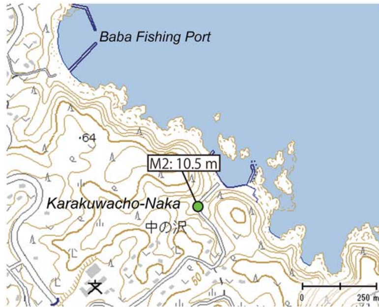
Fig. A135. Tsunami height at Karakuwacho-Naka, Kesenuma City, Miyagi Prefecture (added with a digital topographic map at a scale of 1/25,000 from the Geospatial Information Authority of Japan). The symbol and its meaning are the same as in Fig. 4.
