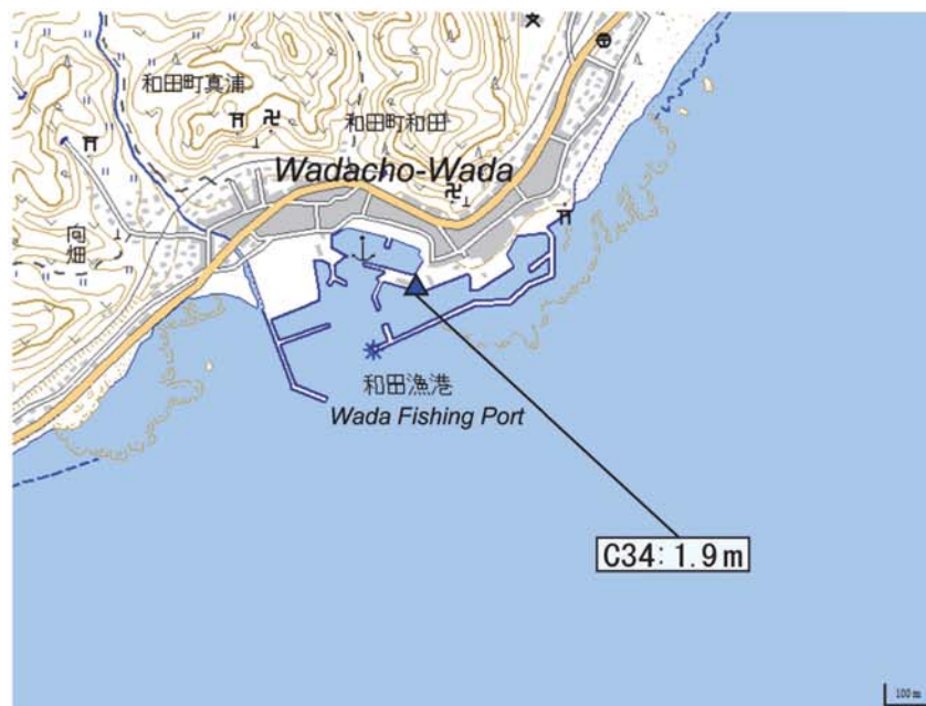
Fig. A341. Tsunami height at Wadacho-Wada (Wada Fishing Port), Minamiboso City, Chiba Prefecture (added with a digital topographic map at a scale of 1/25,000 from the Geospatial Information Authority of Japan). The symbol and its meaning are the same as in Fig. 6.
