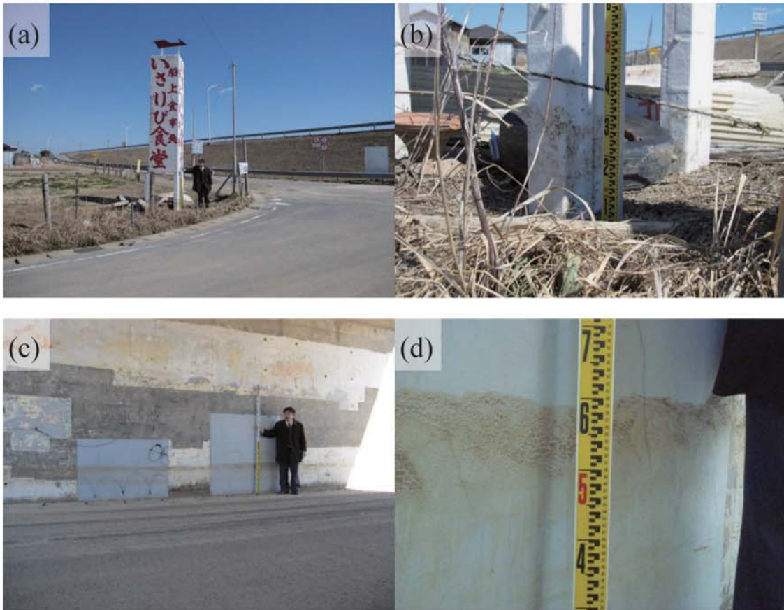
Fig. A316. (a)-(b) Watermark on the prop of a signboard (0.29m above ground level; C16). (c)-(d) Watermark in a tunnel under Kujukuri tollway (0.56m above ground level; C17).
