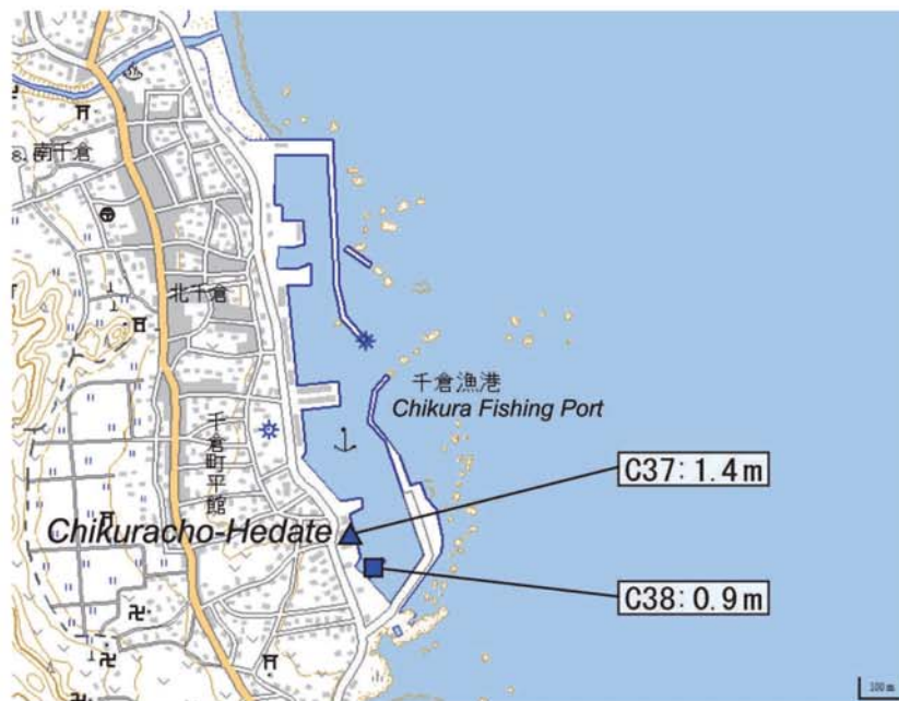
Fig. A345. Tsunami heights at Chikuracho-Hedate (Chikura Fishing Port), Minamiboso City, Chiba Prefecture (added with a digital topographic map at a scale of 1/25,000 from the Geospatial Information Authority of Japan). The symbols and their meanings are the same as in Fig. 6.
