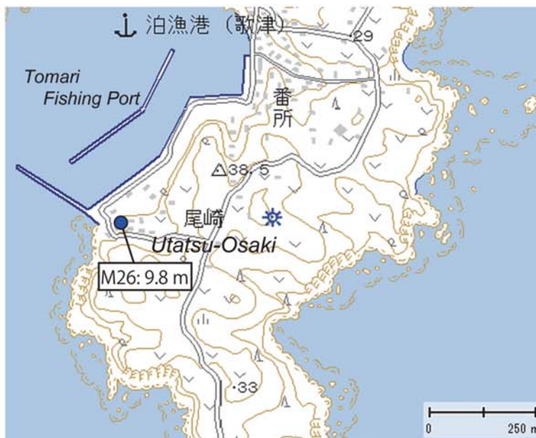
Fig. A161. Tsunami height at Utatsu-Osaki, Minamisanriku Town, Miyagi Prefecture (added with a digital topographic map at a scale of 1/25,000 from the Geospatial Information Authority of Japan). The symbol and its meaning are the same as in Fig. 4.
