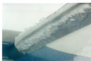
(Fig.2) In-flight icing on leading edge<sup>(1)</sup>
