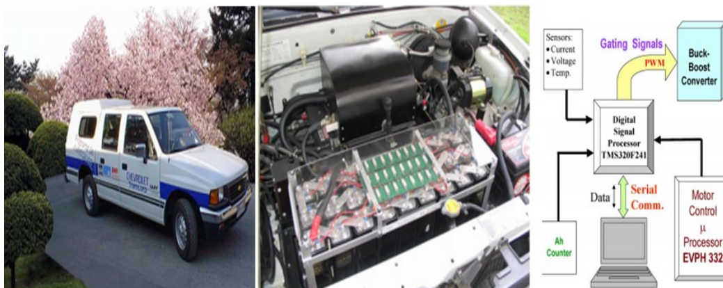
Figure 1.2 Structure of EV with ZEBRA battery and super capacitor hybrid system [6, 7, 8]
