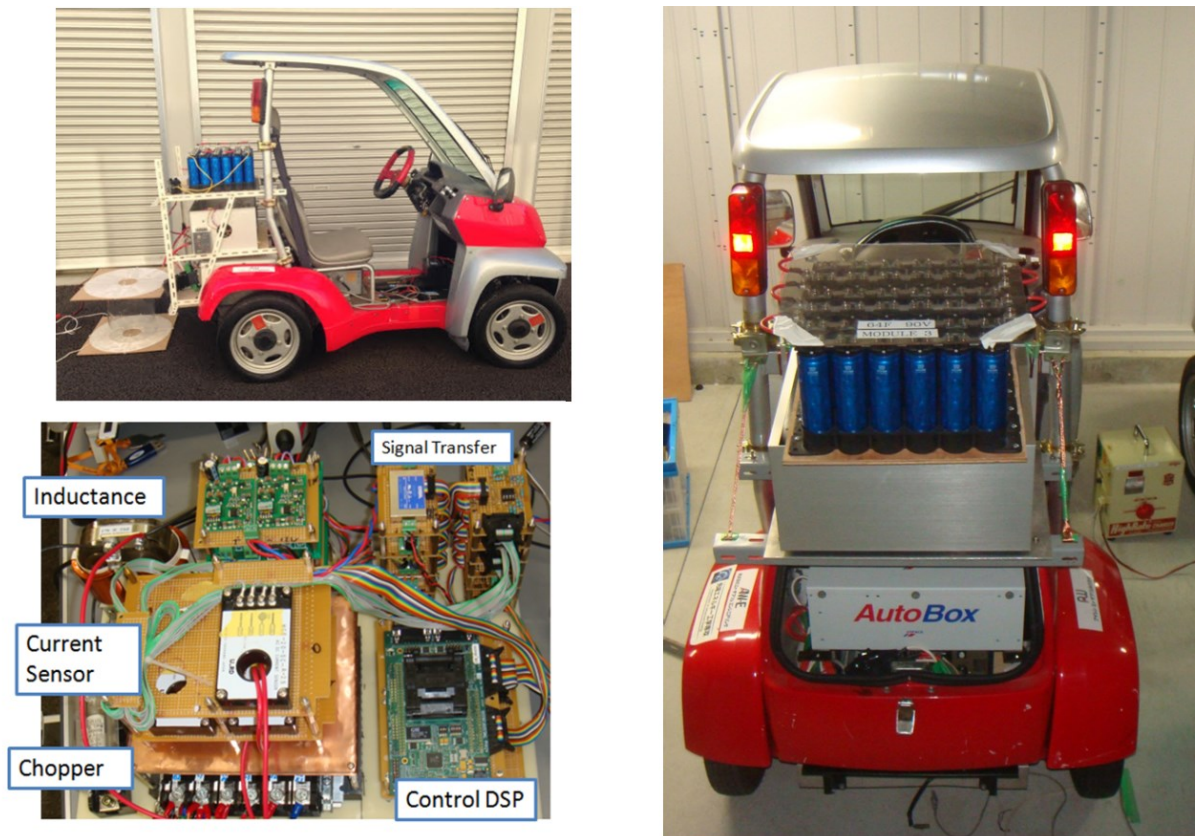
Figure 5.3 Arranged hybrid energy systems for EV prototype
