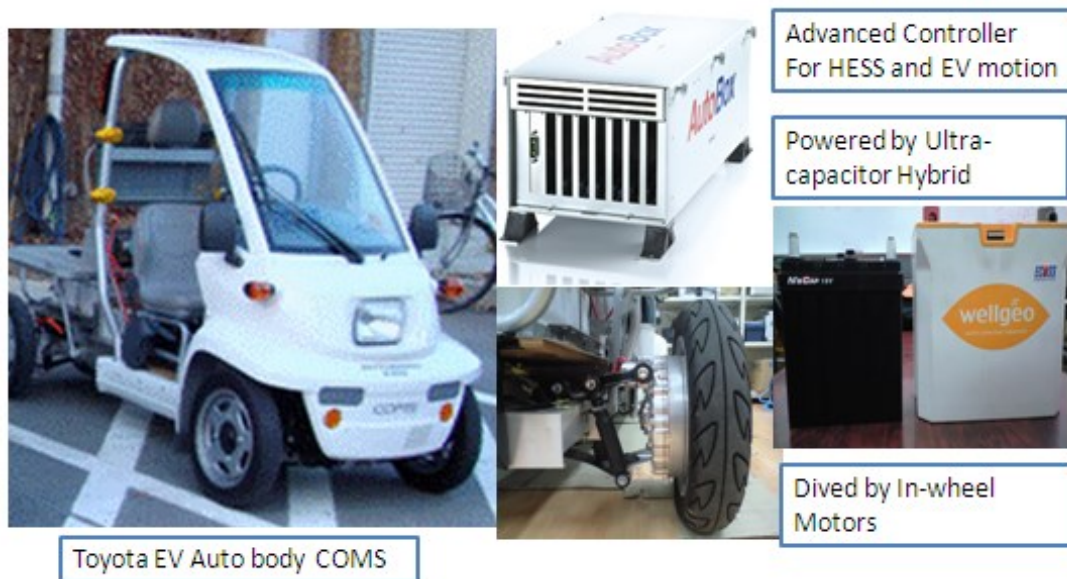
Figure 5.1 Sections of hybrid energy EV CMOS
