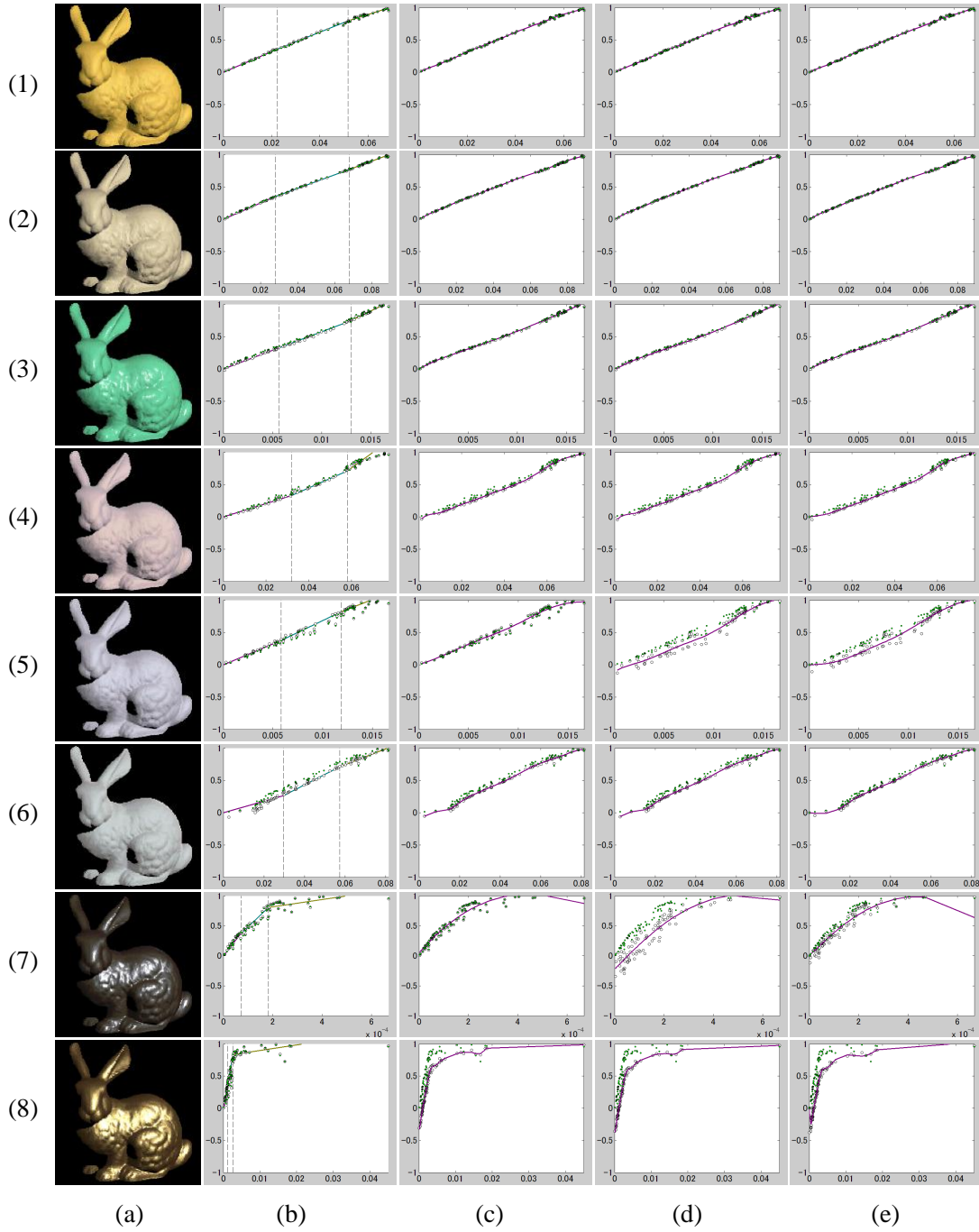
Figure 6-1: (a) Input images (only one pixel is sampled in the experiments), (b)-(e) Recovered 2-d plots ( I_i, \mathbf{n}^T l_i ) (blank circles), function (colored lines) of PL-SBL, NL-LS, NL-SBL and NL-SBL (modified version) with ground truth 2-d plots (green circles).
