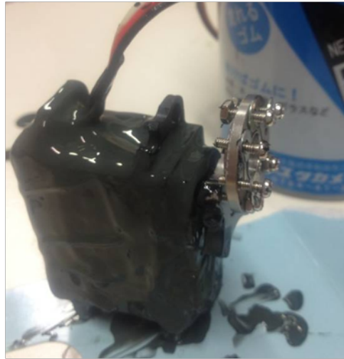
Figure 2.17: Servomotor Gum Protection
