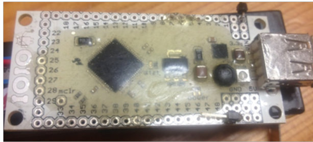
Figure 2.14: IOIO Board Protected With Epoxy
