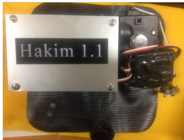
Figure 2.18: Final Airbag System after Waterproofing [19]
