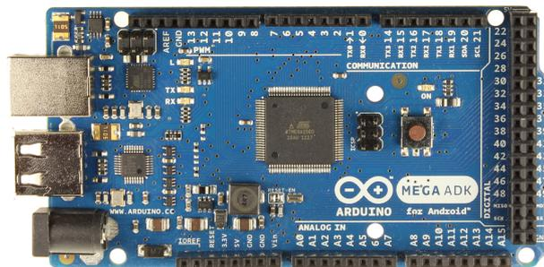
Figura 9: Arduino ADK (ARDUINO, 2014).
