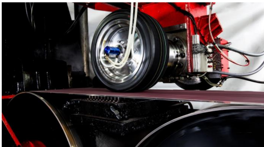
Figura 5-11: Teste de pneu na Calspan [29]
