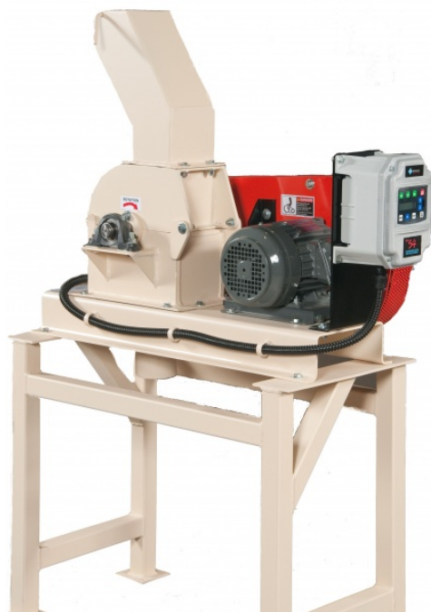
Figura 11- Moinho martelo do modelo W-6-H Series Laboratory Scale Hammer Mill, marca Schutte Buffalo.
