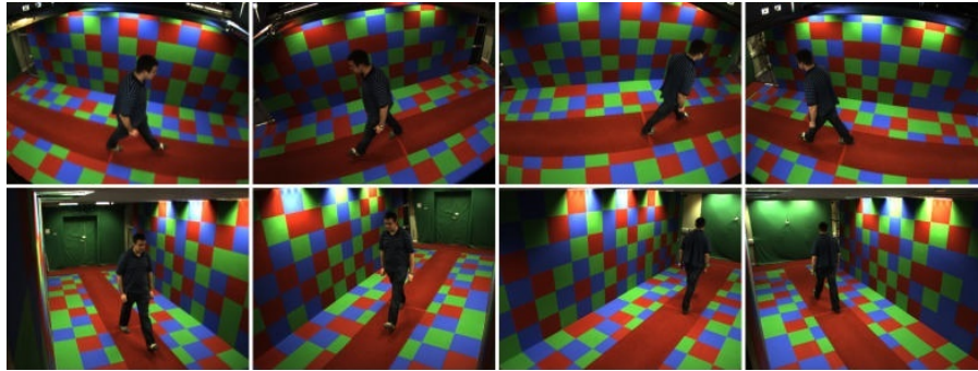
Figure 2.12: Gait images captured by the synchronized cameras in the multi-biometric tunnel of University of Southampton [64].
