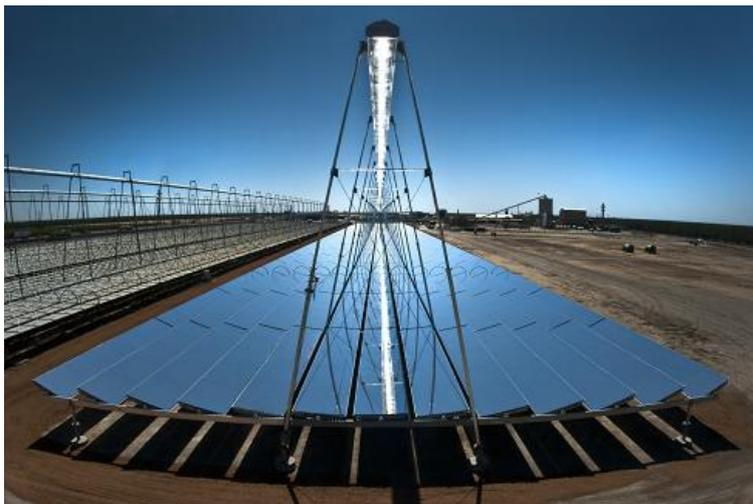
Figura 12- Refletor Linear Fresnel. Fonte: <[www.climateactionprogramme.org/climate-case-studies/the\\_future\\_of\\_concentrating\\_solar\\_power/](http://www.climateactionprogramme.org/climate-case-studies/the_future_of_concentrating_solar_power/)> Acesso em maio 2014.
