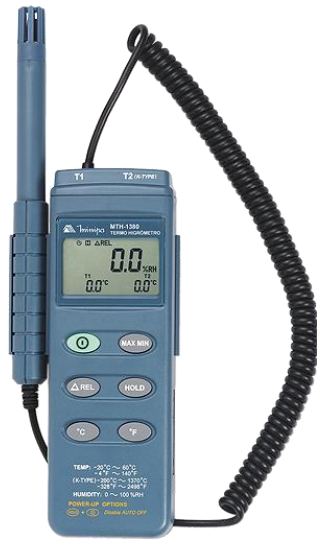
Figura 23: Termohigrômetro Minipa MTH-1380 (Minipa, 2012).
