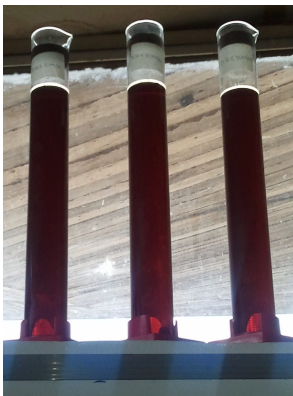
Figura 12 - Amostras das misturas 2 – (a) D30E20M50, (b) D30E30M40, (c) D20E30M50
