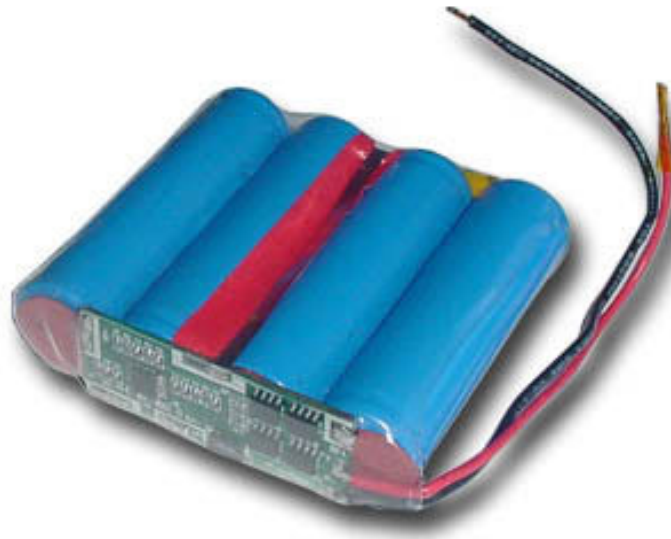
Fig. 3.3. Individual battery pack with protection circuit.
