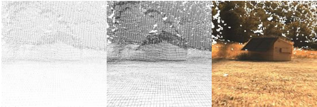
Fig. 1.1. Lidar x-y-z point cloud, wire mesh and textured 3d image.
