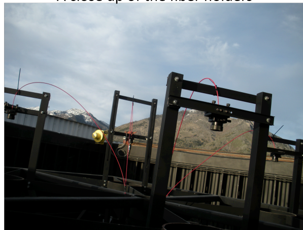
A close up of the fiber holders
