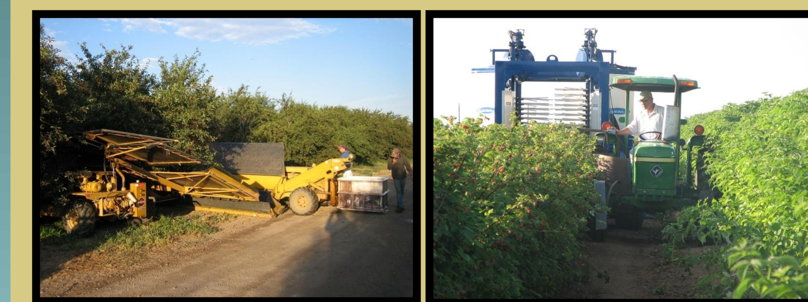
Figure 6. Existing mechanical harvest technology includes tart cherry harvester (Santaquin, UT) and a raspberry harvester (Laketown, UT)
