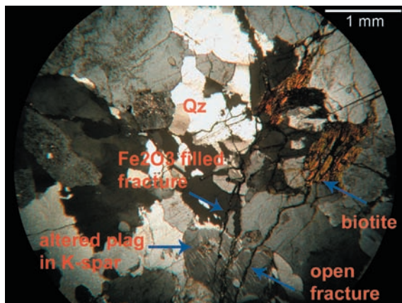
Figure 5. Photomicrograph in cross polarized light of the Grass Valley fault zone hanging wall 1 m from the fault core. Note the pronounced decrease in damage from Figure 4 (Jacobs, 2005).
