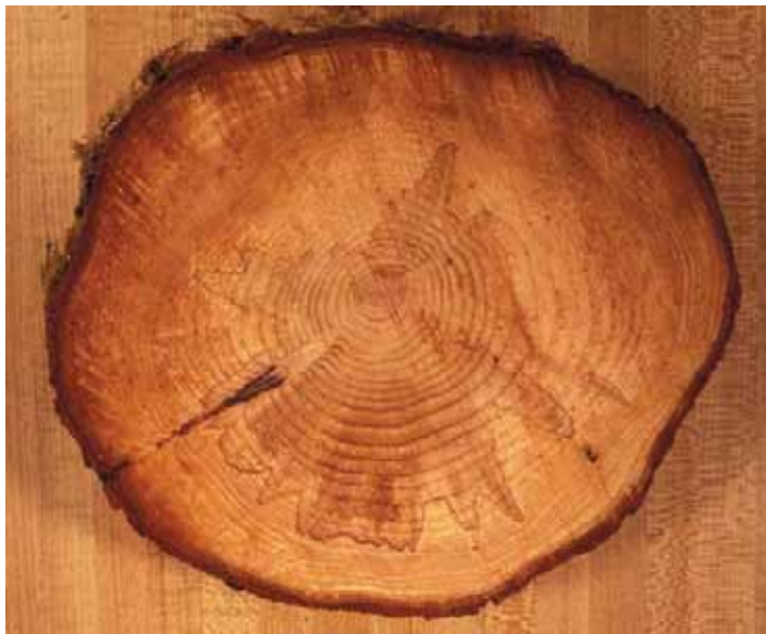
Figure 7 —Common staining and decay caused by Heterobasidion annosum as it appears in a cross section of hemlock. (Photo courtesy of W.G.Thies)
