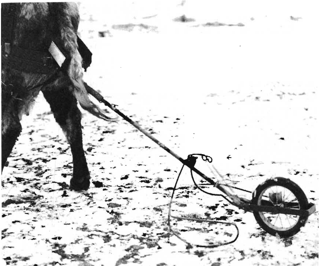
Figure 8. A range meter to measure the distance traveled by cattle.
