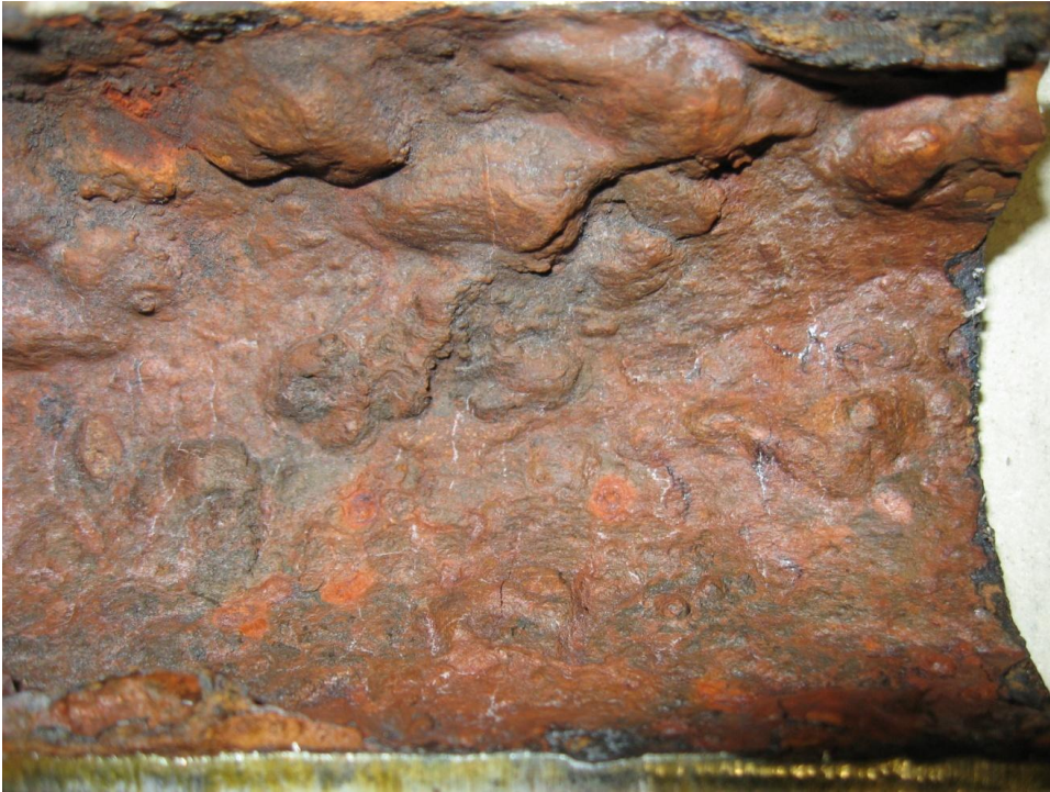
Figure 11: Photograph of the longitudinally cut 0.050-m aged pipe
