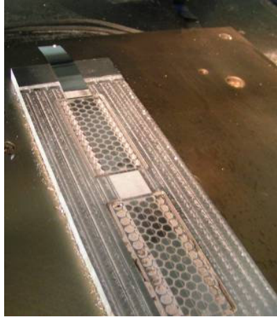
Figure 15. Test specimen for thermoset support material, with honeycomb lattice.
