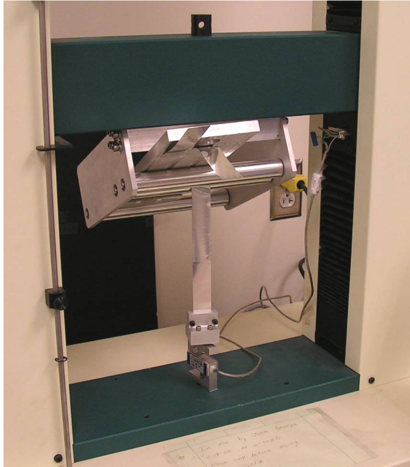
Figure 9. Loaded peel test apparatus with 4 inch plate and three consolidated tapes.
