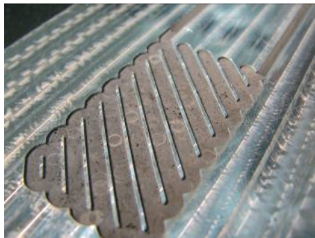
Figure 16. Test specimen for contamination-free support material experiment.
