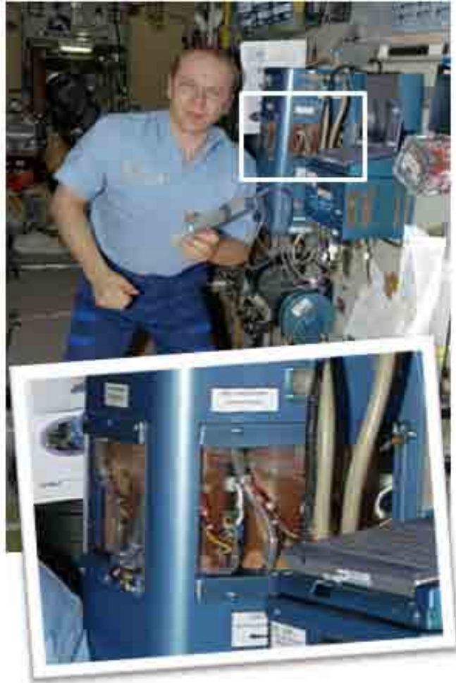
Fig. 3.3: Cosmonaut Oleg Kotov priming the experiment with water on the International Space Station in July 2007. The porous media were launched oven dry. Air in the tubes and porous membranes was replaced with water through manual Cosmonaut intervention facilitating the first wet-up of the porous media in the process. An automated procedure then continued to wet up the media to a matric potential of -2 \text{ cm}_{H_2O} and subsequently drained the media to a potential of -30 \text{ cm}_{H_2O} , at which point the automated experiments began. The cut-out shows heterogeneous wetting patterns observed in Turface, Mix and Profile during priming, leaving behind dry clusters of media.
