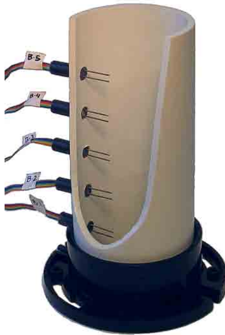
Fig. 4.3: Plant-growth column used in the stratified porous-media root zone experiments. The 25 cm tall column allows hydration via the establishment of a shallow saturated zone at the bottom of the root zone using a small port at the base. The inside look shows the possible placement of integrated dual-probe heat-pulse sensors amenable for the estimation of water content and electrical conductivity.
