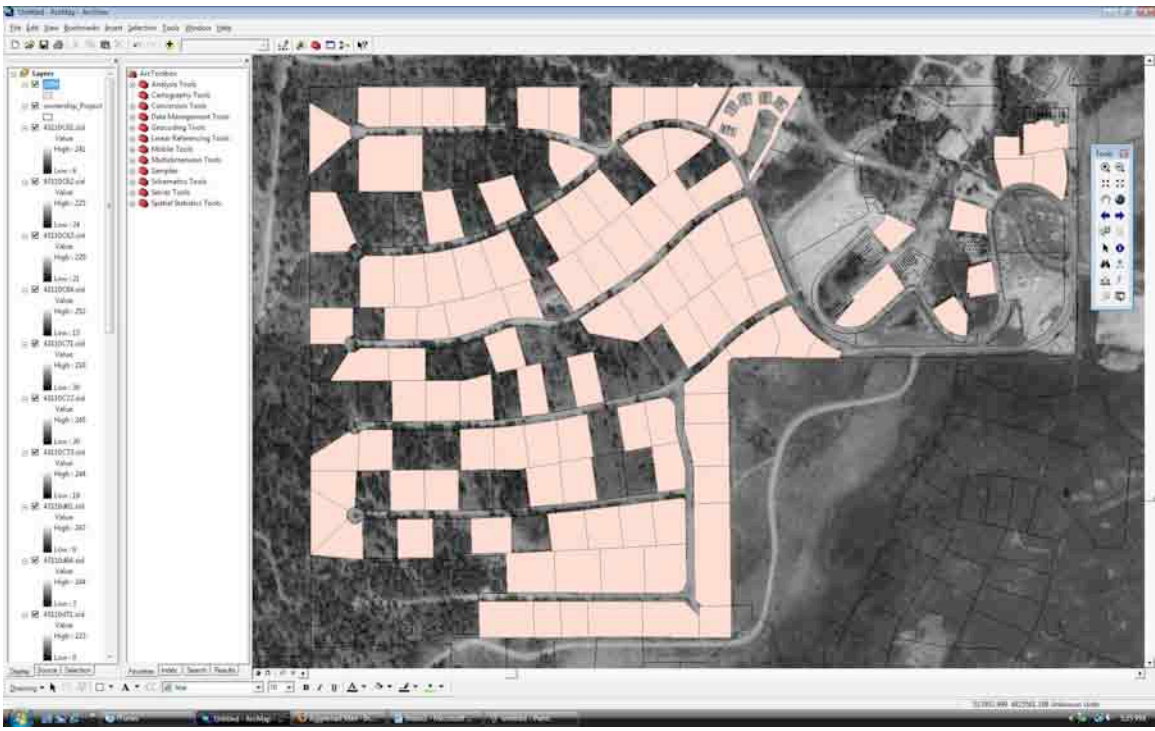
Figure 2-8. Exporting selected parcels to create a new layer that represents parcels with new development.
