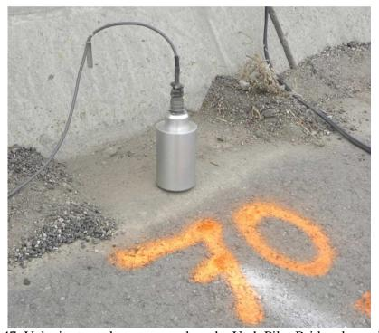
Figure 47. Velocity transducers as used on the Utah Pilot Bridge dynamic test.
