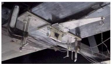
Figure 17: Deflectometer on bottom flange of a girder.
