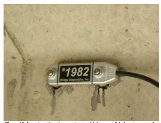
Figure 19. Location of strain transducer at highest possible location on web.
