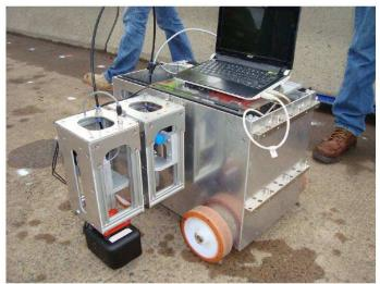
Figure 7: Performing impact-echo testing.
