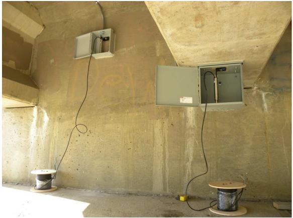
Figure 54. Showing two tiltmeters installed one on girder and one on abutment.
