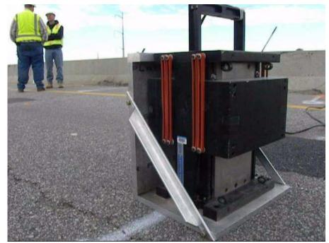
Figure 46. Electromagnetic shaker used in Utah Pilot Bridge dynamic test.
