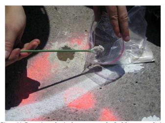
Figure 11: Removing pulverized concrete samples for laboratory analysis.
