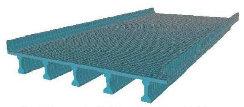
Figure 9: 3-D representation of the bridge model using Frame and Shell elements.
