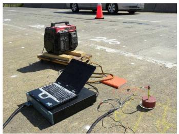
Figure 13: Measuring reinforcing steel corrosion rates.
