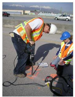
Figure 10: Pulverizing concrete samples with a hammer drill.
