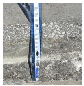
Figure 6. Measurement of asphalt overlay thickness.
