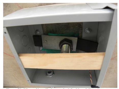
Figure 70. View of installation method for hitec foil strain gauges.
