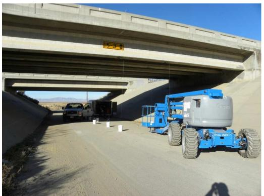
Figure 20. Boom lift and weights used to provide initial deflection for "Twangers."
