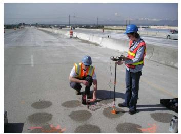
Figure 12: Conducting half-cell potential testing.
