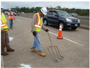
Figure 5: Performing a chain drag test.
