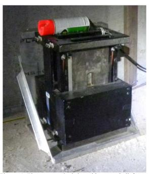
Figure 19: Electromagnetic shaker with custom built frame.
