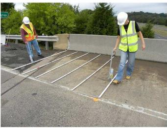
Figure 3: Marking a grid pattern or deck testing.
