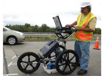
Figure 6: Conducting a ground penetrating radar survey.
