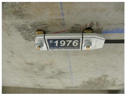
Figure 11. Surface mounted strain transducer, showing identification number.
