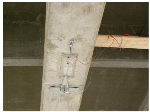
Figure 18. Strain transducer at bottom flange and Twanger at midspan.
