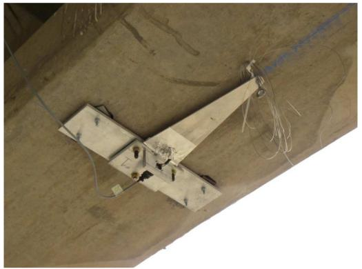
Figure 12. Deflection instrument, "Twanger."
