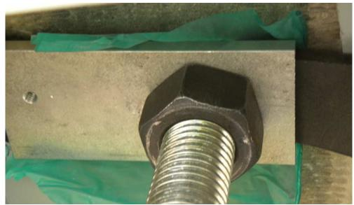
Figure 71. Close-up view of installation method for vifoil strain gauges.
