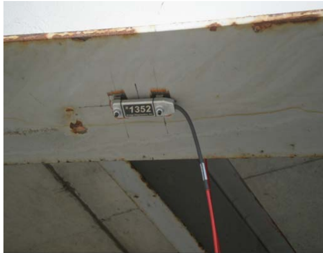
Fig 3.17 Typical strain gage used in the live load test.
