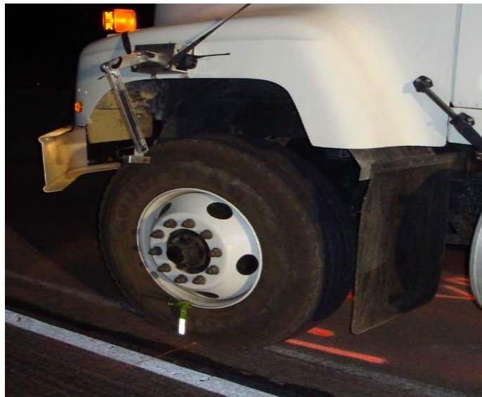
Fig 4.14 Auto-clicker mounted on the test truck.
