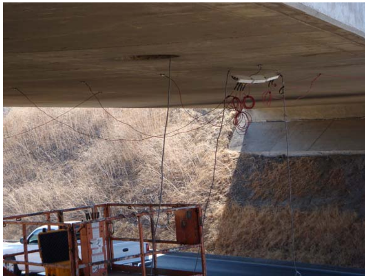
Fig 4.9 Part of the BDI structural testing system (STS).
