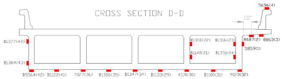
Fig 4.12 Sensors ID and locations for Section DD. (Courtesy of BDI).
