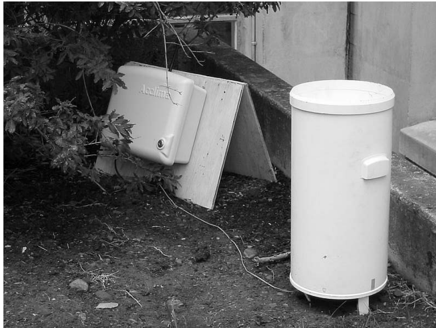
Fig. 6.1: Final DataManager product with enclosure actively measuring precipitation and soil water content at a USU test site.
