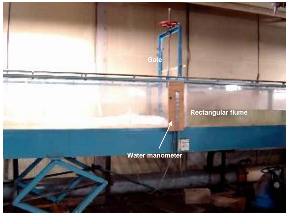
Fig. 6. Rectangular flume, sluice gate, and manometer board
