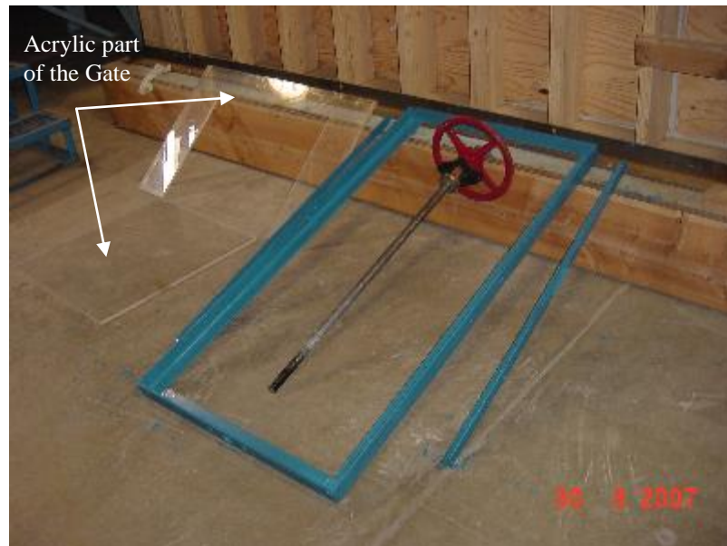
Fig. 39. Parts of the gate before to installation in the flume
