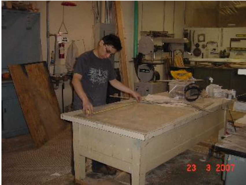
Fig.37. Construction of the vertical sluice gate
