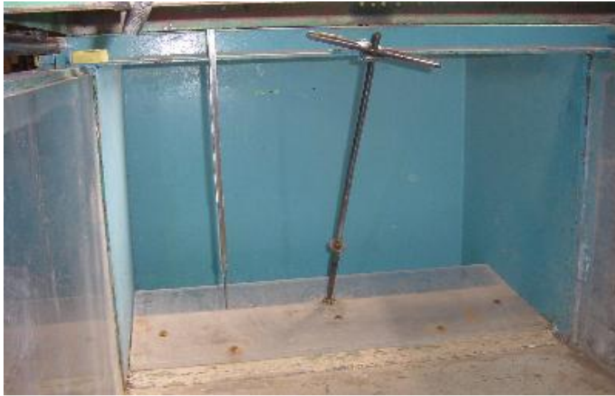
Fig. 4. Photograph of the downstream of the flume with a tailgate to control the water depth downstream of the sluice gate
