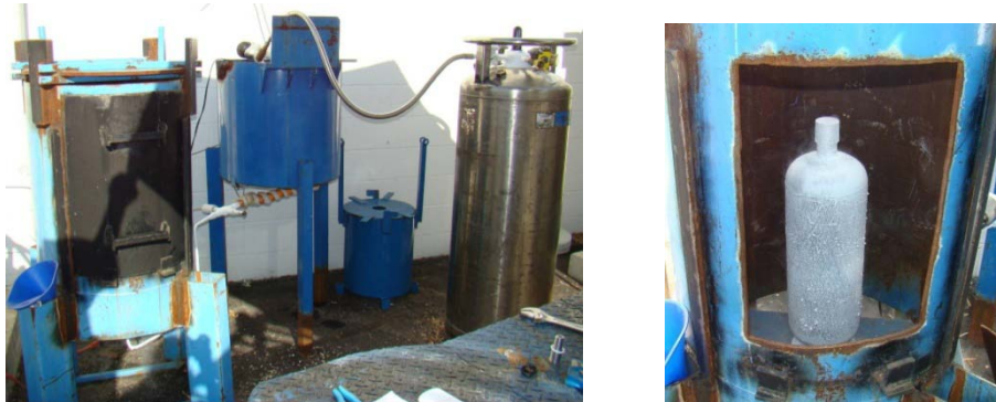
Figure 13. The left image illustrates the cryogenic test setup located at HEI's test facilities in Brigham City, UT. The image on the right shows a vessel that has just undergone the autofrettage process.
