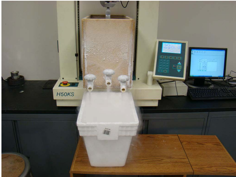
Figure 18. The image above illustrates the improved cryostat that was designed to allow the NOL test rings to be submerged in LN 2 during the tensile tests.
