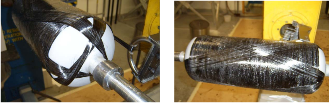
Figure 12. Filament winding of the buckling test specimens.
