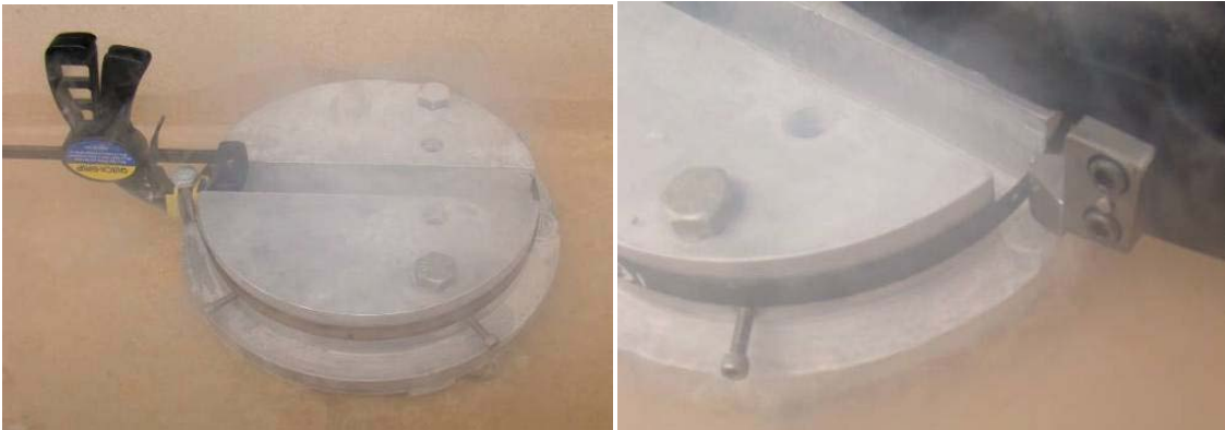
Figure 15. Modified Charpy impact test anvil.
