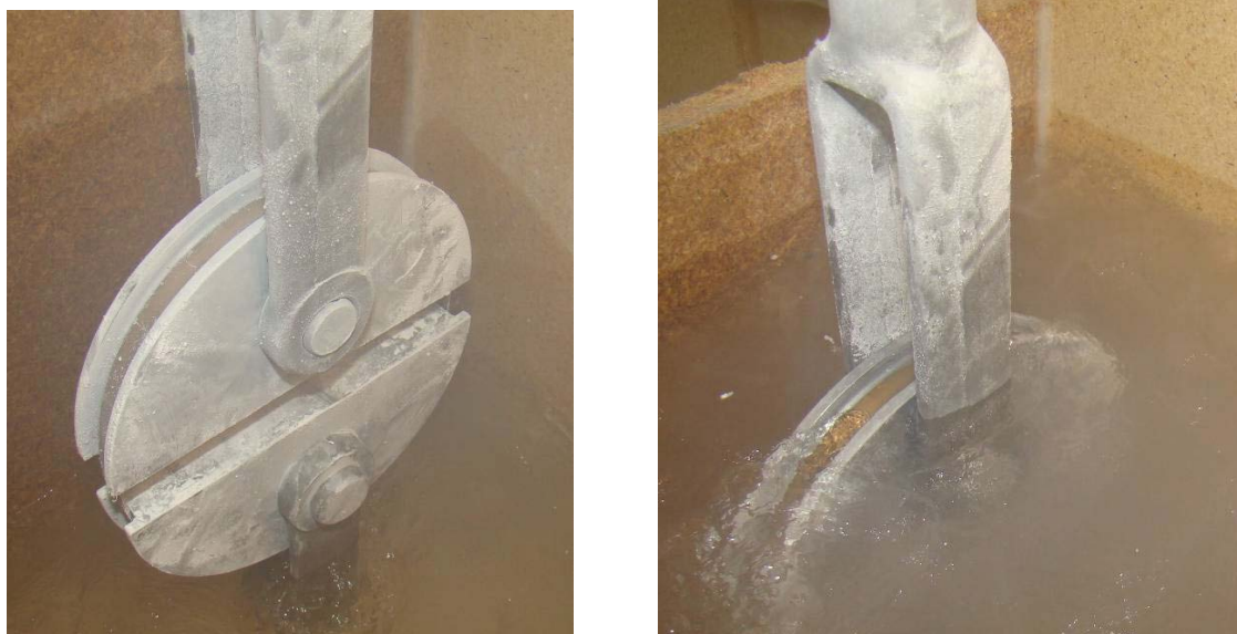
Figure 19. The images above show the NOL ring loaded on the split disk fixture ready for testing.
