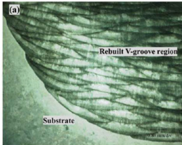
Figure 11. Picture shows the rebuilt area and substrate. The microstructure of the rebuild can also be seen (Song et al., 2006).
