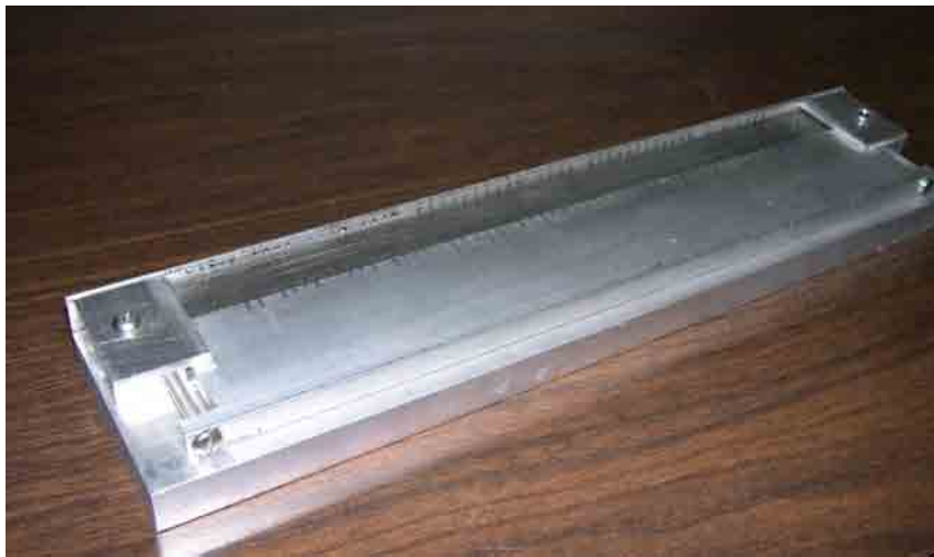
Figure 14. The large fixture used to produce the samples for the initial and final phases.
