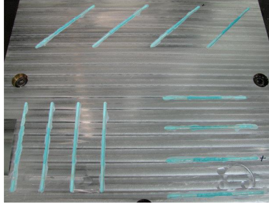
Figure 3.31: Experiment setup for embedding using channels.
