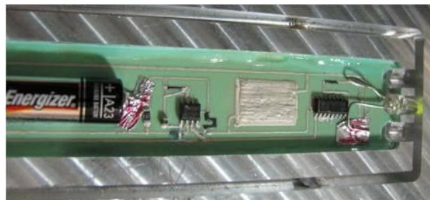
Figure 4.11: Touch sensor circuit with lid LED.
