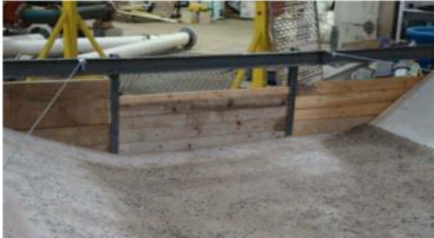
Figure A5. Stop logs installed on the downstream end of the model to set flow depths (Rahmeyer et al. 2010).
