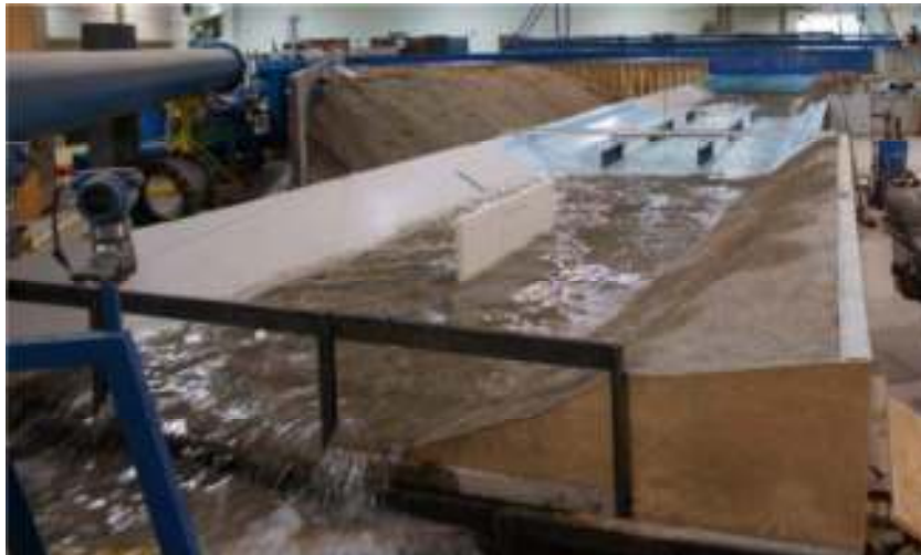
Figure A4. Upstream view of the entire model showing the Wright Street Bridge pier in white in the foreground (Rahmeyer et al. 2010).
