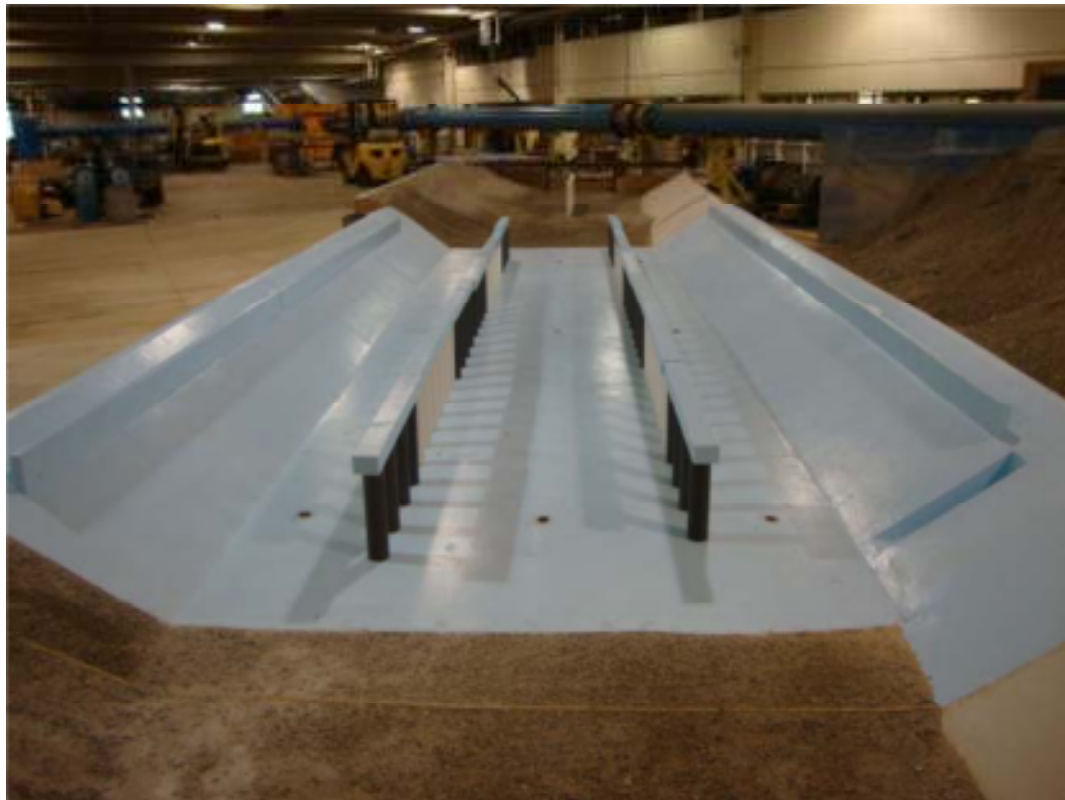
Figure A2. I-84 bridge crossing section looking downstream. Original columns are white and the new columns are black (Rahmeyer et al. 2010).
