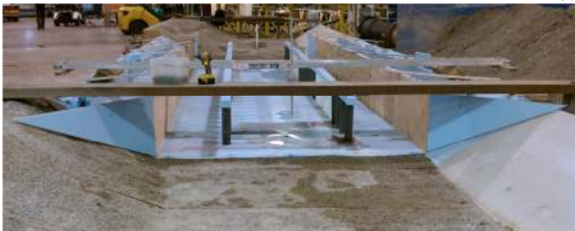
Figure A7. Downstream view of the vertical section with the approach walls installed.
