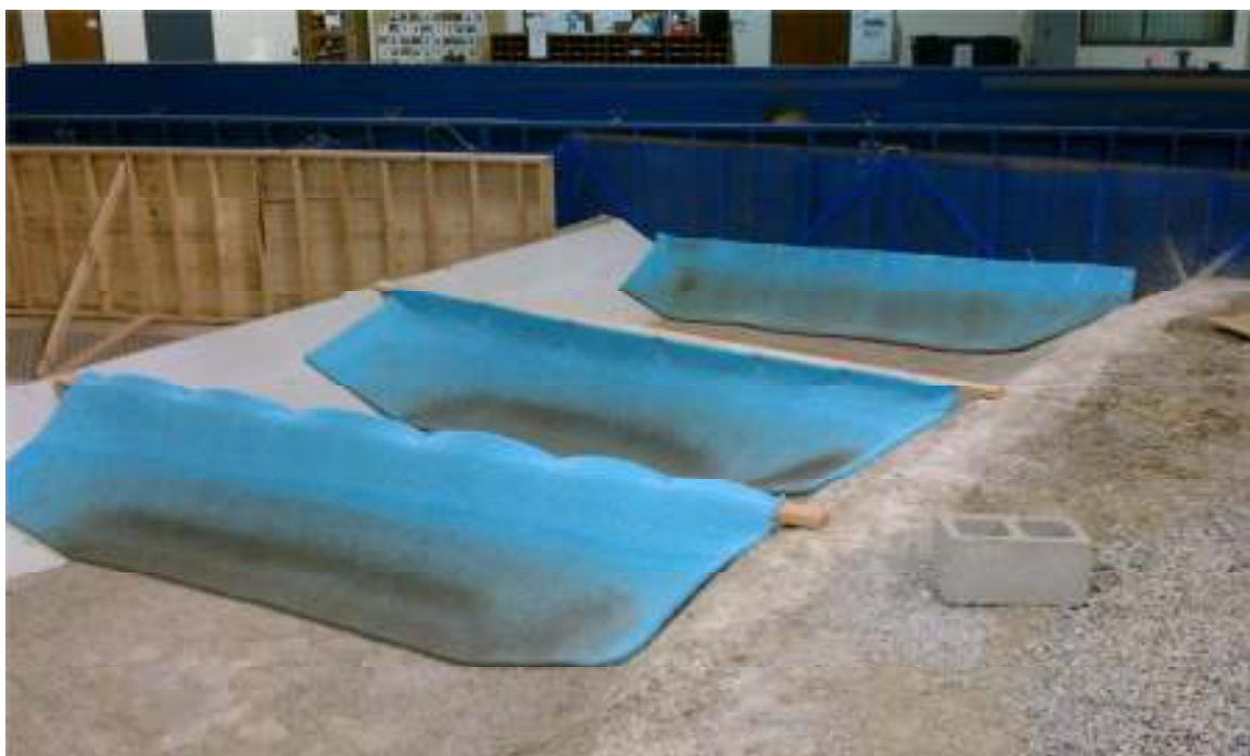
Figure A8. Upstream view of baffles which helped control approach conditions into the model.
