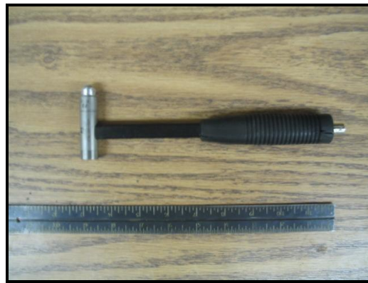
(a) Large instrumented hammer
