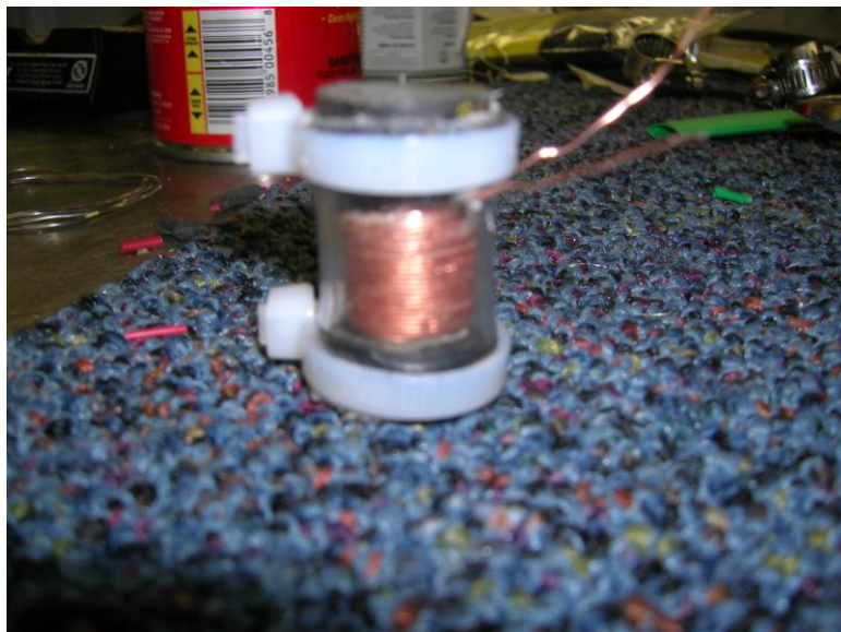
Fig. 5.5. Plastic tube housing
