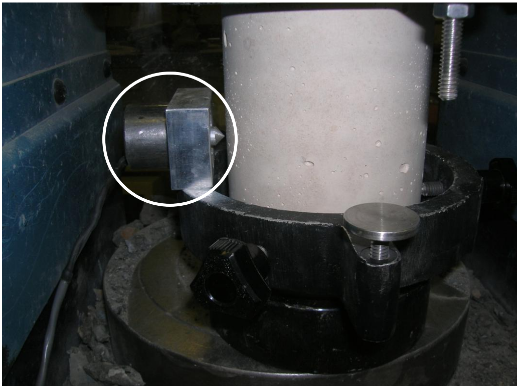
Fig. 5.9. Excitation device mounted on side (in circle)
