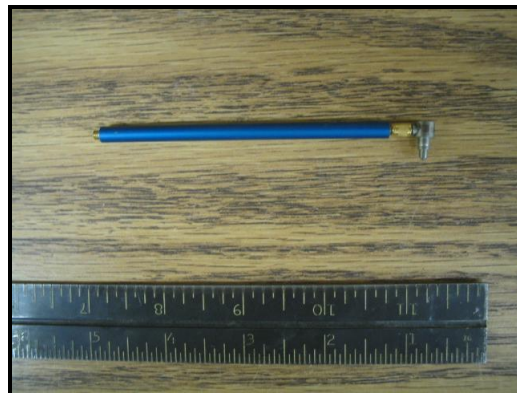
(b) Small instrumented hammer
