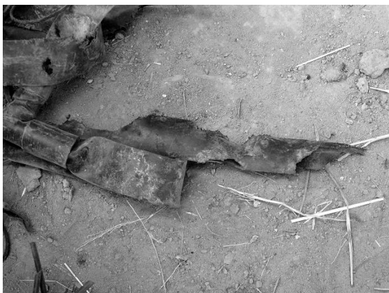
Fig. H.27. Drip system eaten by rats while in storage. AG3.
