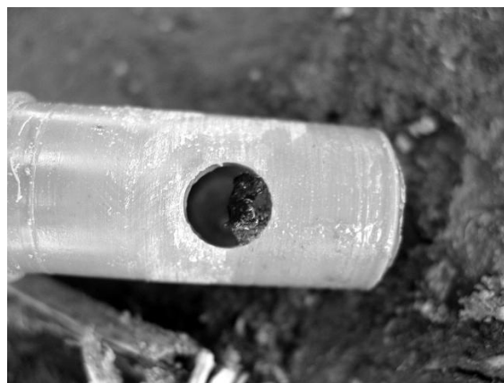
Fig. H.12. Debris in the valve stopcock. EC3.
