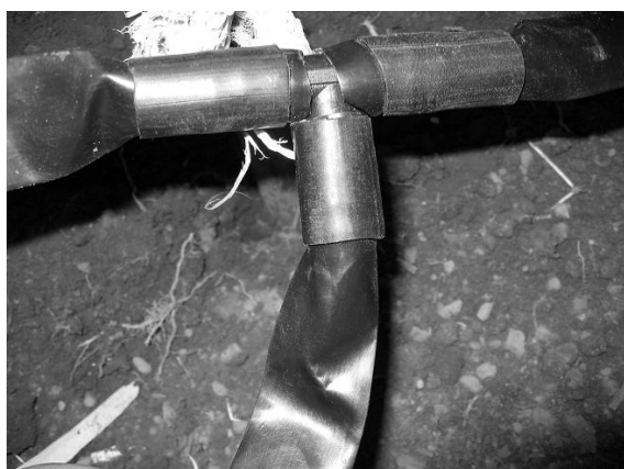
Fig. H.39. Lateral attached crooked and folded. Golba3.
