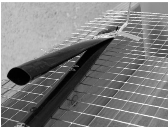
Fig. B.9. Lateral end plug by folding the lateral
