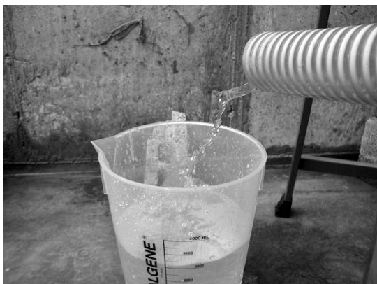
Fig B.3. Volumetric method for flow measurement
