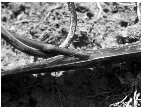
Fig. H.25. Emitter inserted into the edge of a twisted lateral. SDS.
