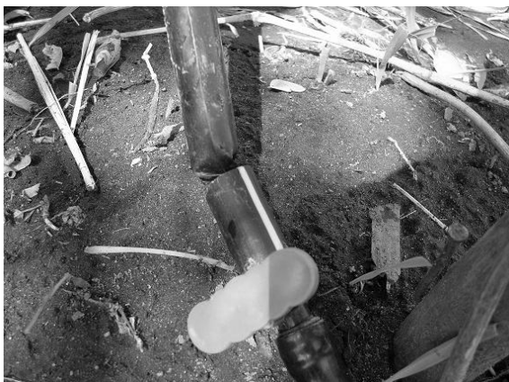
Fig. H.7. Kink in the mainline at the connection with the valve. EC1.
