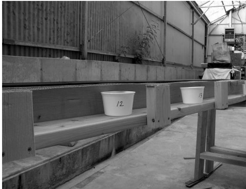
Fig. 1. Testing runway. The runway included wire mesh to support the lateral and a shelf for the catch cups (two of which are shown here).
