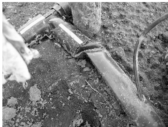
Fig. H.8. Kink in the lateral at the connection with the submain. EC1.
