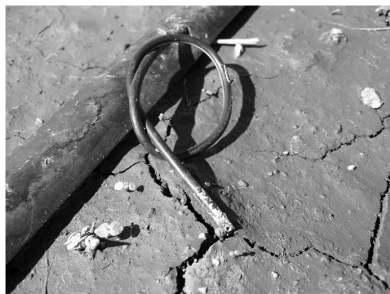
Fig. H.16. Emitter outlet lying in the soil. EC4.
