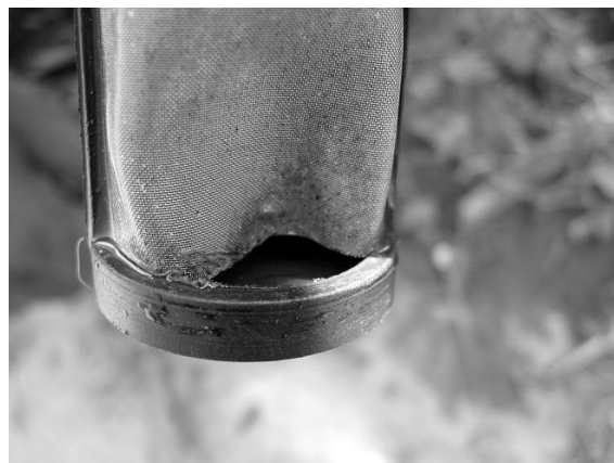
Fig. H.28. Tear in the filter screen. AGFTC.
