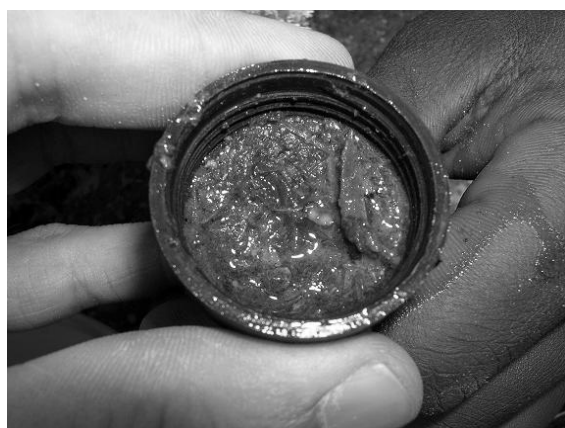
Fig. H.4. Clogged inline filter. EC1
