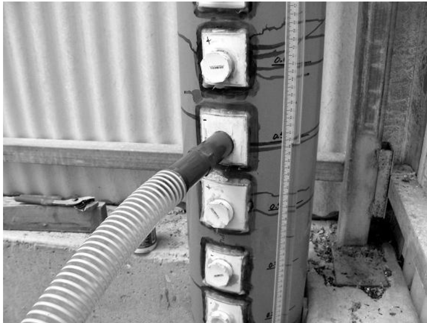
Fig. 2. Downstream tank. The overflow holes were tapped to facilitate flow measurement.
