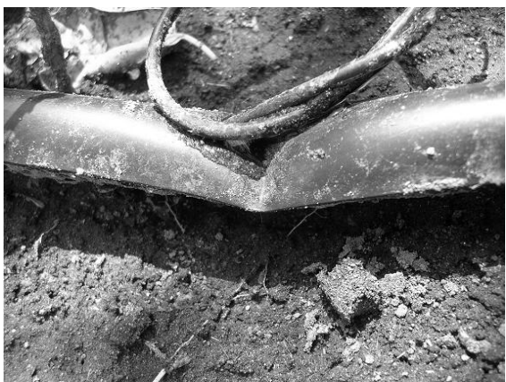
Fig. H.5. Kink in the lateral due to microtopography. EC1.
