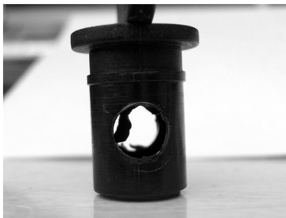
Fig. B.13. Valve stopcock debris before cleaning
