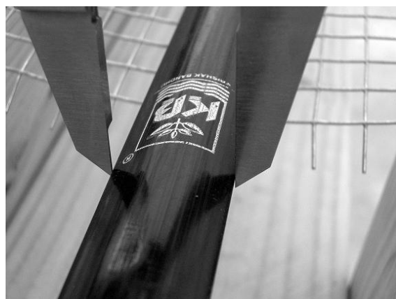
Fig B.6. Lateral cross-section measurement using calipers
